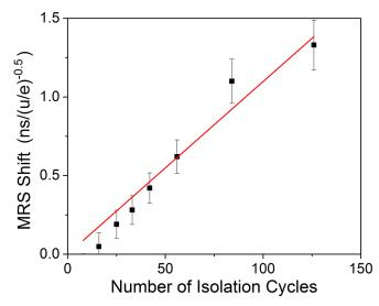
FIG. 9. Measured shift of the time of flight of  $^{133}$ Cs ions due to the MRS as a function of the number of isolation cycles. The shift is normalized by  $(m/q)^{1/2}$  (for details, see text). The lines show a fit of Eq. (13) to the data points. The resulting fit constant is  $A_{\rm mrs} = 1.1 \times 10^{-11} \ {\rm s}/\sqrt{{\rm u/e}}$ .
