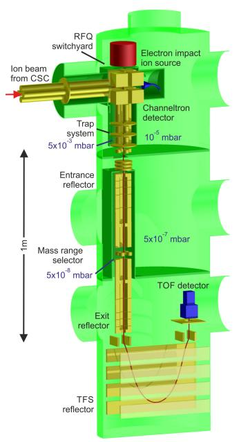
FIG. 3. Schematic figure of the multiple-reflection time-of-flight mass spectrometer. The ions enter from the CSC in gas-filled radio-frequency quadrupoles. They are mixed with ions from the calibration sources and are cooled and bunched in a system of linear RF traps. From here, they are injected in the TOF analyzer.
