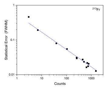
FIG. 11. Statistical uncertainty normalized to the FWHM of the peak as a function of the number of measured  $^{213}$ Fr ions per spectrum of experiment I. The mean value for the FWHM of the distribution in this measurement was  $1.03 \times 10^{-3}$  u/e.
