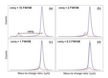
FIG. 1. Schematic mass-to-charge spectra illustrating the four classes of close-lying peaks as defined in the text. The distances between the mass distributions are 10, 2, 1, and 0.3 FWHM for classes A to D, respectively. The peak shape and the abundance ratio of 1 to 10 is selected to be identical for all classes. The thin black curves show the sum of both distributions.
