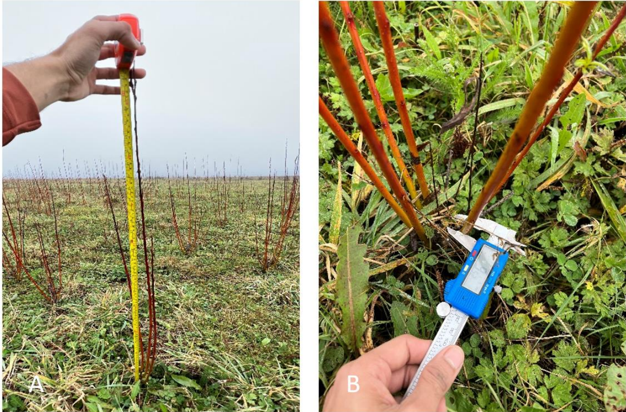
Figure 3.10.2.2.2 Measuring trees stem length (A) was measured using a measuring tape, and stem diameters were measured using a vernier caliper (B).
