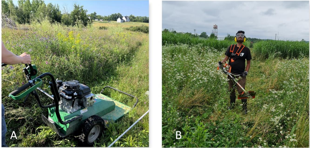
Figure 3.9.1 A self-propelled brush cutter used to mow weeds around subplots (A) and handheld brush cutters used to control weeds within the tree subplots (B).
