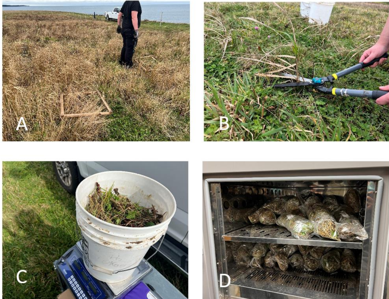
Figure 3.10.2.1.1 Grass sampling using shows the (from left) 0.25 m 2 quadrants at the Chegoggin Point site (A). Harvesting aboveground biomass of miscanthus (B). A biomass sampled being weighed at the site (C) and drying of the sub-samples in the drying oven in the lab.
