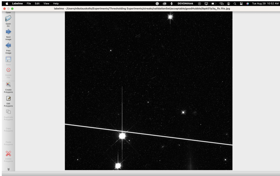
Figure 4.3: The labelMe image annotation software being used to create pixel-level annotations of satellite trails in HST images.
