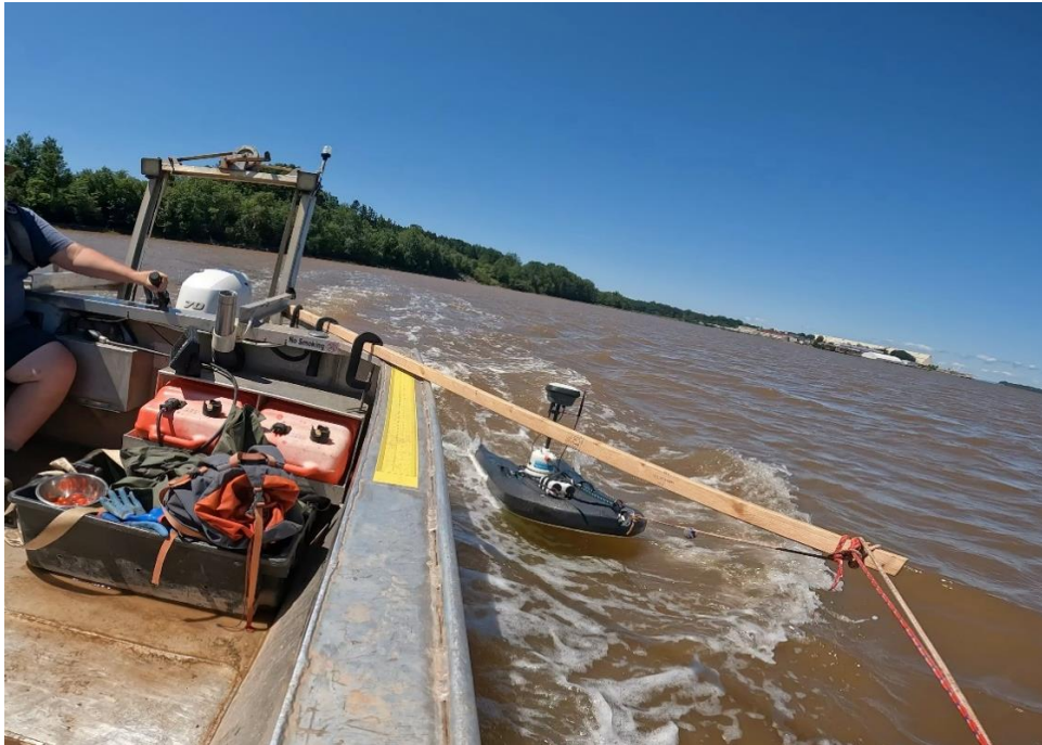
Figure 3.1 M9 ADCP attached to a fishing boat to complete the bathymetric surveys along transect lines.
