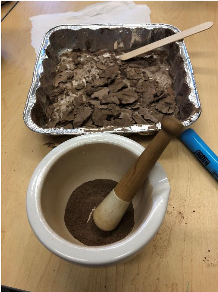
Figure 3.7: Sediment samples dried in aluminum trays then powdered using a mortar and pestle.
