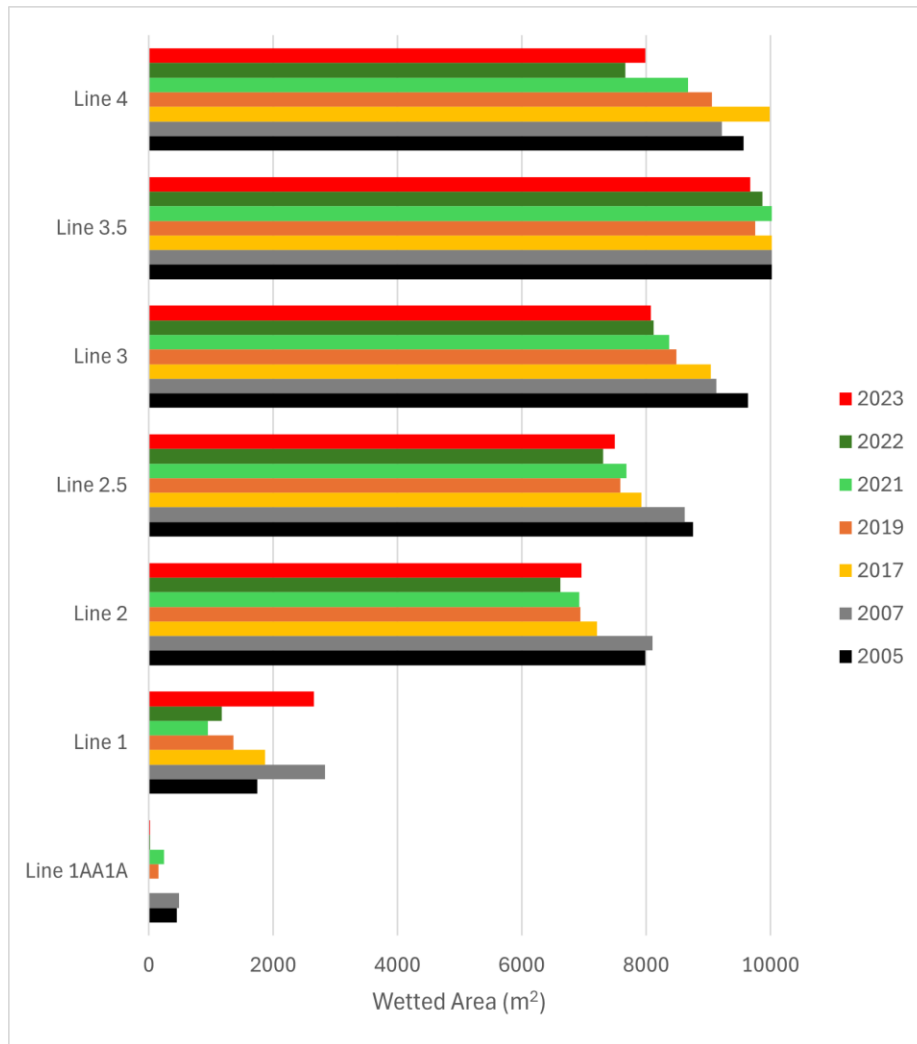
Figure 4.4: Wetted area of the Avon River, lines closest to the causeway are at the bottom of the figure while lines furthest away are at the top.
