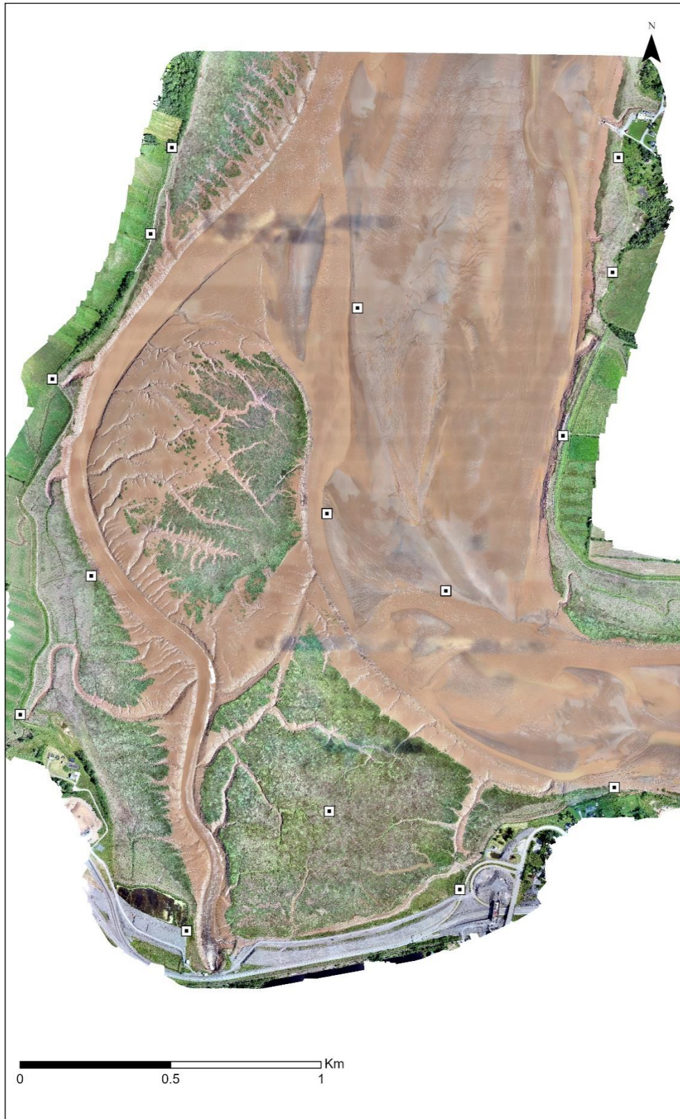
Figure 3.2: Locations of GCPs deployed during RPAS. Base image is the orthomosaic collected during RPAS on August 4th, 2023, basemap provided by ESRI Canada.
