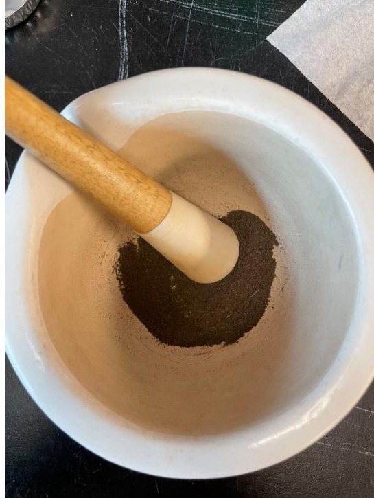
Figure 26. Grinding and homogenization of soil sample with mortar and pestle.
