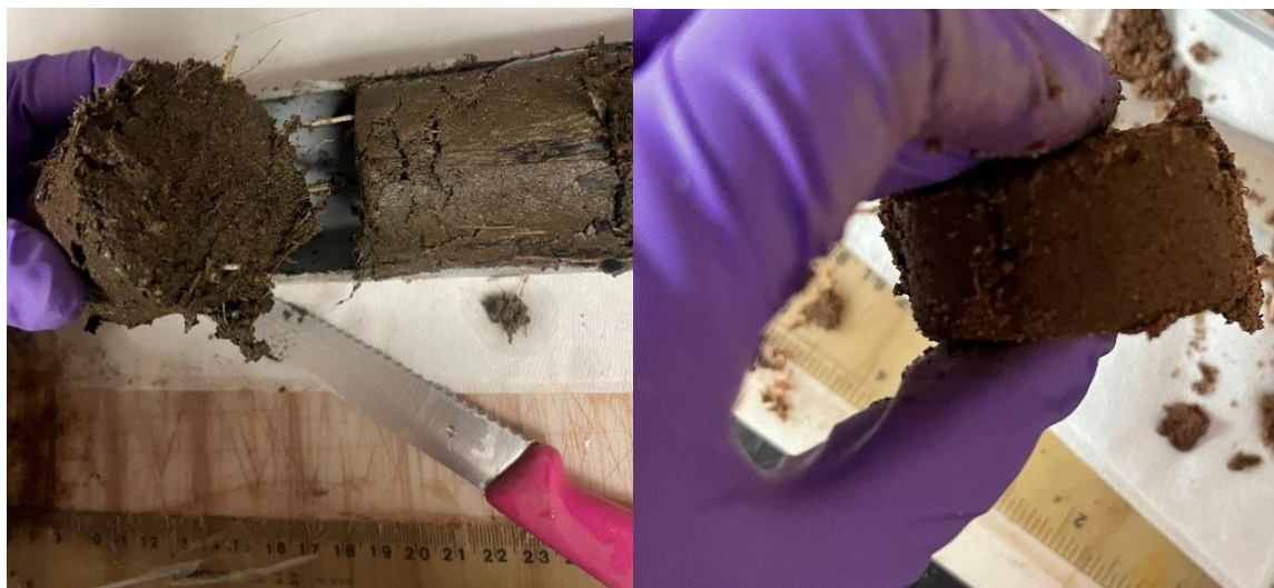
Figure 25. Bulk density disc cut out of sediment core sample
