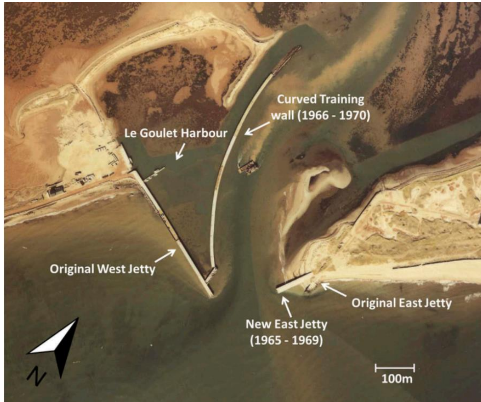
Figure 10. Historical engineering works at Shippagan Gully from the late nineteenth century to the mid-twentieth century (photo taken in 1980) (Provan et al., 2018).
