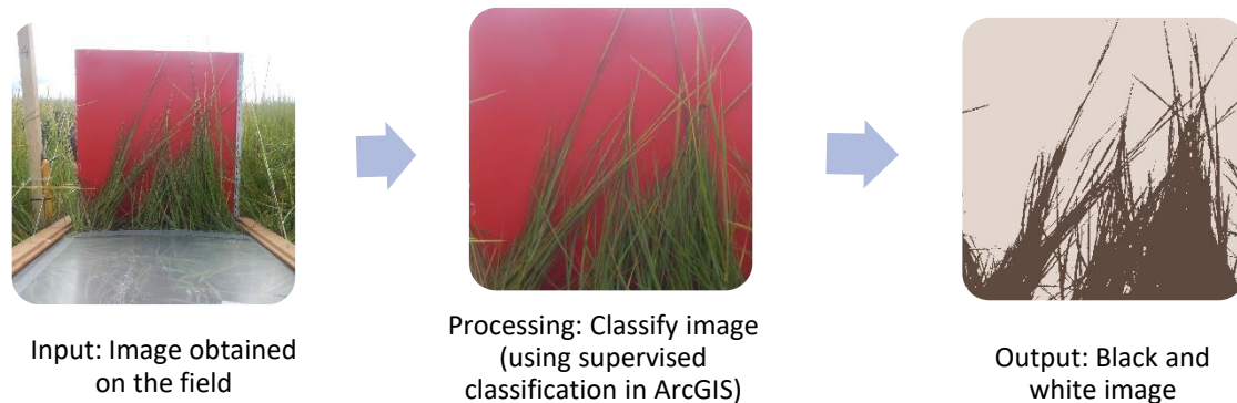
Figure 20. Schematic diagram illustrating how to derive obscuration ratio (black pixel coverage (%) of image) and canopy height from field image, to classified image and classified binary black and white image.
