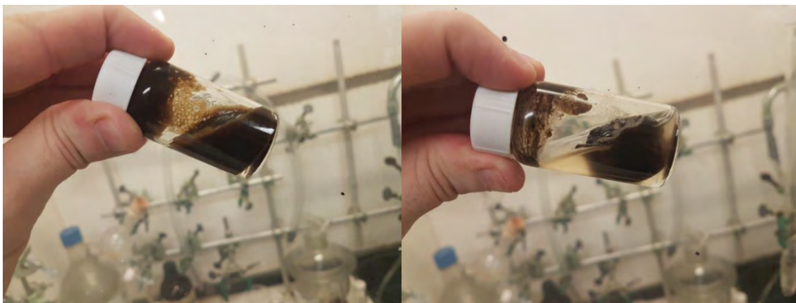
Figure 18: Demonstration of the “gelling” effect of bitumen in water left in the dark.
