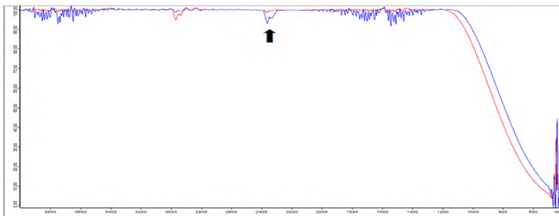
Figure 38A: Infrared spectra for the gases above a photo-oxidized sample of weathered AWB bitumen run in a sealed quartz cell, before exposure to sunlight (red) and after being exposed to sunlight for 3 h (blue).
