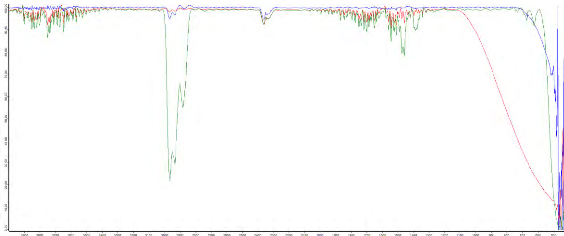
Figure 42: Infrared spectra for the gases above photo-oxidized samples of three bitumen samples after 3 h of sun exposure, for scale comparison only: AWB bitumen (red), weathered AWB bitumen (blue), AWB bitumen + 1% w/w hemin (green).
