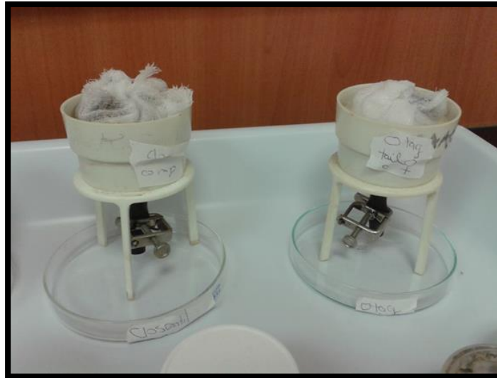
Figure 6: Baermann Funnel used to recover active larvae from faeces.
