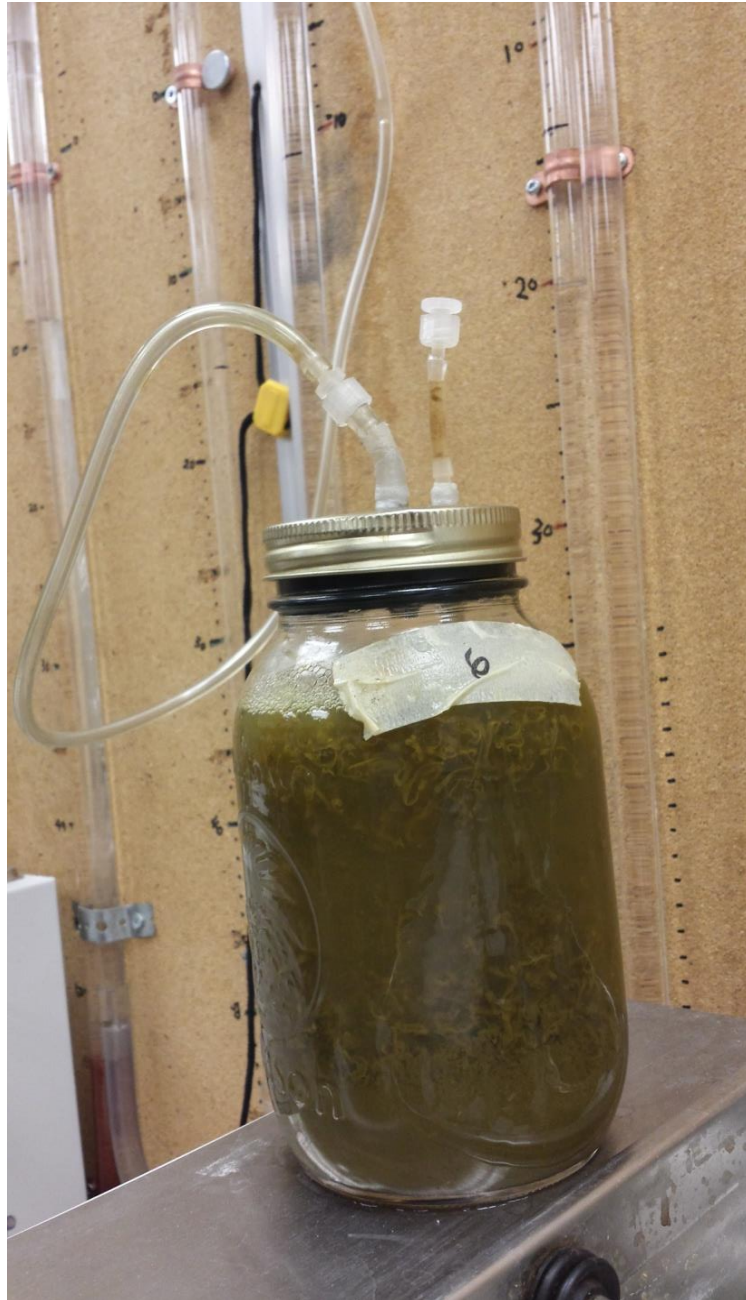
Figure 2.4 Digester jars. The digester jars contained different types and states of engineered wood products and diluted cow manure and kept them in water bath at 39°C.
