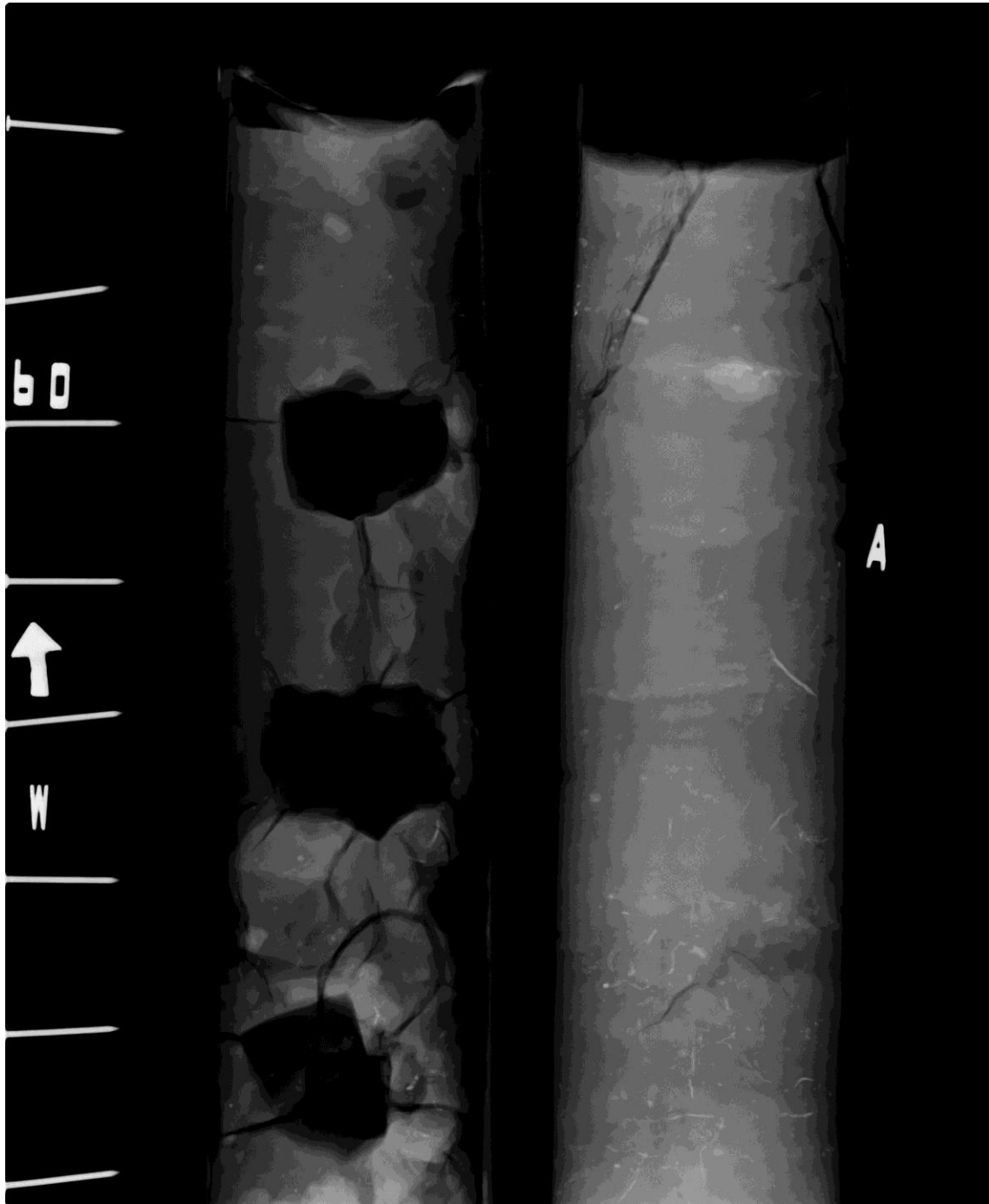
Fig. B-16 – X-radiograph showing iron monosulphides as described in text
