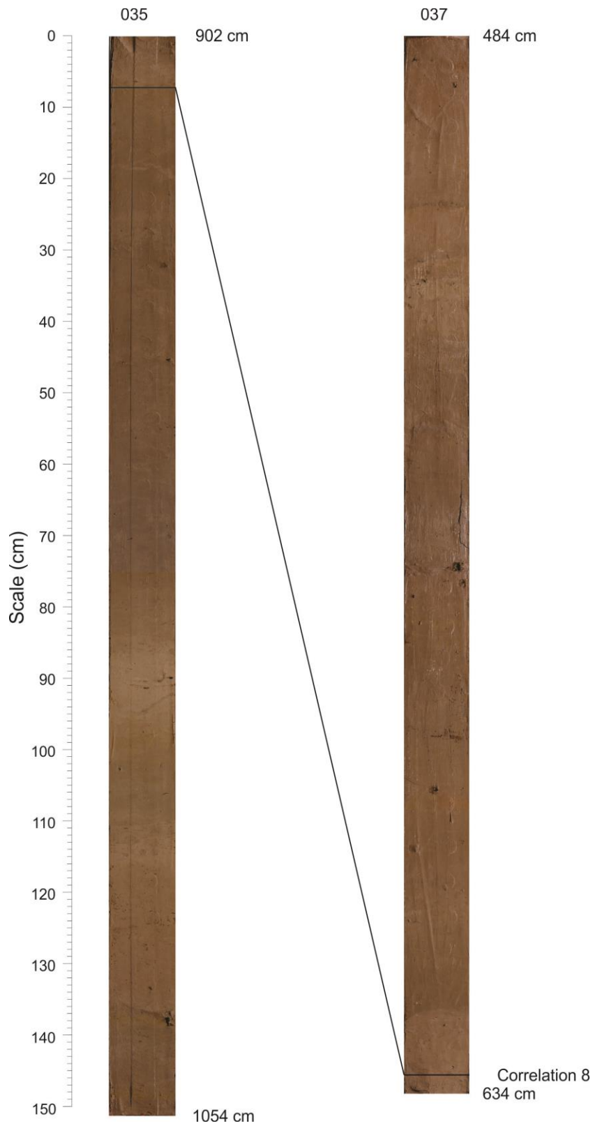
Fig. A-5 – Correlation 8 between piston cores 35 and 37 depicted on core photography
