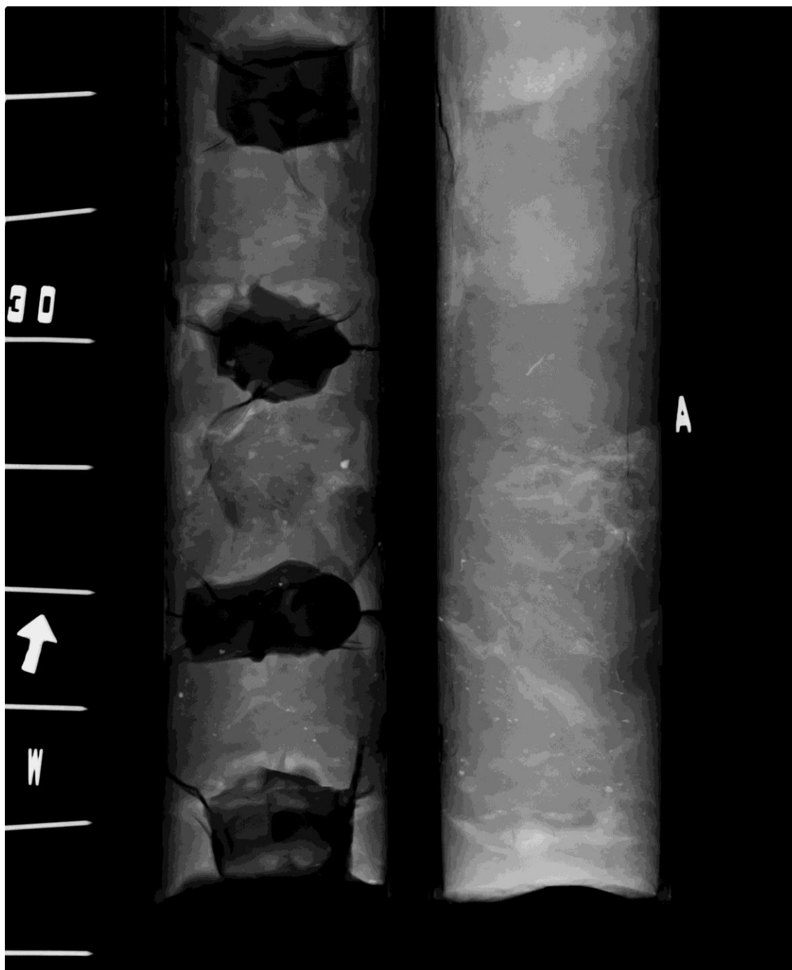
Fig. B-15 – X-radiograph at 30 cm showing bioturbated interval as described in text
