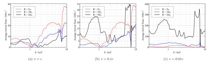
Figure 9. The average arrival times (relative to the earliest arrival of photons in each case) of photons as a function of energy after a luminosity fluctuation propagating radially outwards through the corona at varying radial velocity v. Coronae are considered of different radial extent, R, over the surface of the accretion disc and are located between 1.5 and 2  $r_g$  above the disc plane.
