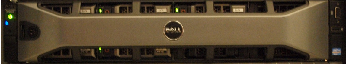
Figure 12: Image of a Dell PowerEdge R720xd piece of equipment
