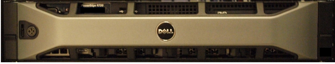
Figure 18: Dell PowerEdge R720 with ignorable regions filled in black (top-middle and bottom-right)
