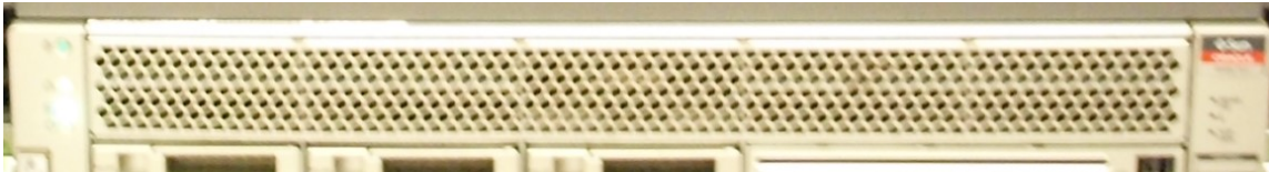
Figure 28: Example of a grill faceplate, Sun server
