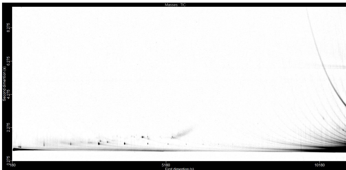
Figure 2.2 A blank GC×GC-FID chromatogram. Black dots at the bottom of the chromatogram are septa bleed. Streaking along the bottom is the solvent peak. Arching lines across the right-hand side of the plot is column bleed. These chromatographic artifacts represent interferences that complicate the calculation of chromatographic complexity using fractal dimensions.
