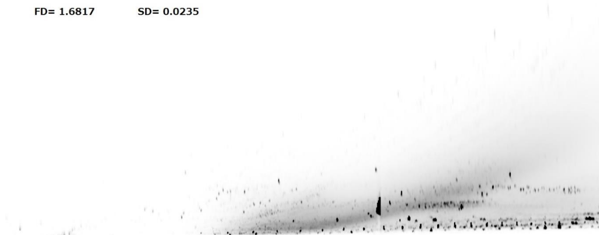
Figure 3.9 GC×GC-FID chromatogram presenting granularity, the granularity in the chromatogram is caused by either a bad run in the GC×GC test or by interference of other elements during the test; granularity makes the fractal dimension increase.
