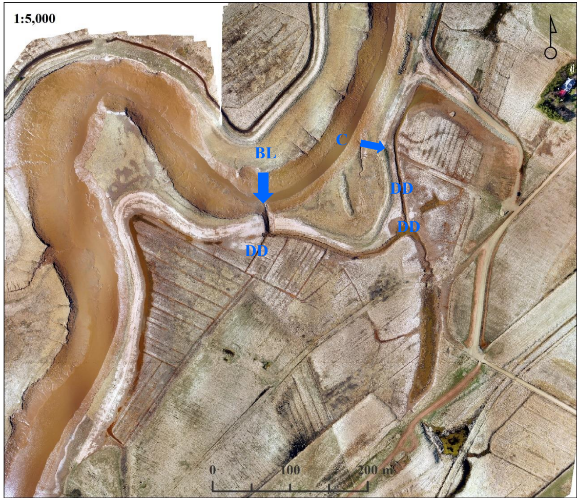
Figure 2.6: RPAS orthomosaic of Converse collected on May 5, 2019 (RPA model: DJI Phantom 3 Professional; flight altitude: 90 m). The breach location (BL) is visible and the levelled sections of the dyke in the south-eastern and most northern end. Former drainage ditches (DD) were also widened, and the culvert (C) was removed. More details on restoration activities are detailed in text. The survey took place for the post-breach classification analysis. (Credit: Akyol, R., Saint Mary's University)
