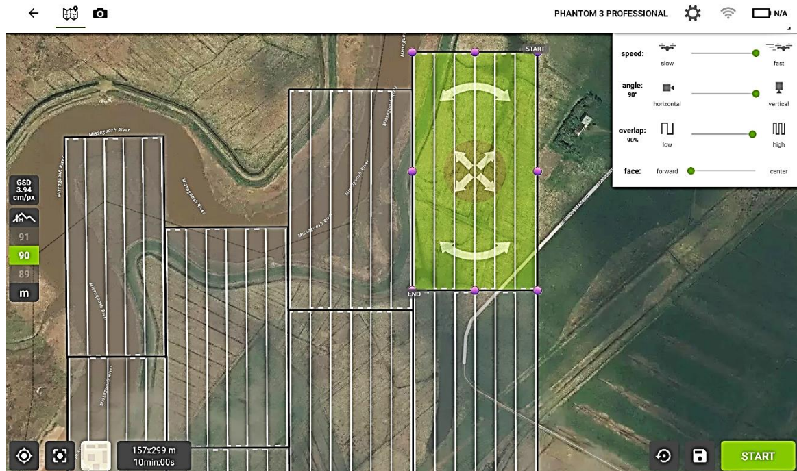
Figure 3.3: RPAS mission plan display, with flight grids superimposed over software basemap of the Converse study area. Display view provides information about flight altitude, ground sample distance, selected grid size with approximate flight time, relative speed and overlap settings (Source: Converse Project in Pix4Dcapture).
