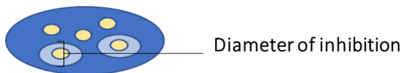
Figure 9. Graphical representation of well diffusion assay extracts against P. larvae (dark blue). Average radius of inhibition can be calculated from average diameter of area of inhibition (pale blue). Average radius = Average diameter/2
