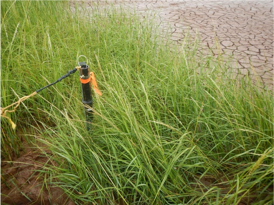
Figure 3.3. Location and set-up of Level logger at the marsh edge. Photo taken on August 17, 2020.
