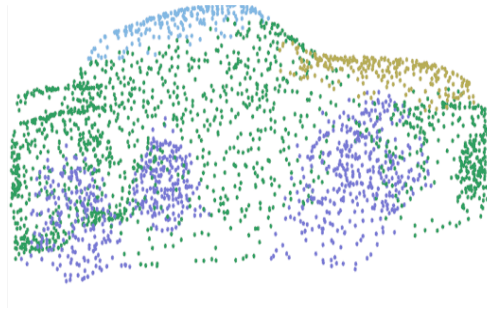
Figure 1.4: An example of unordered point cloud scan [8].
