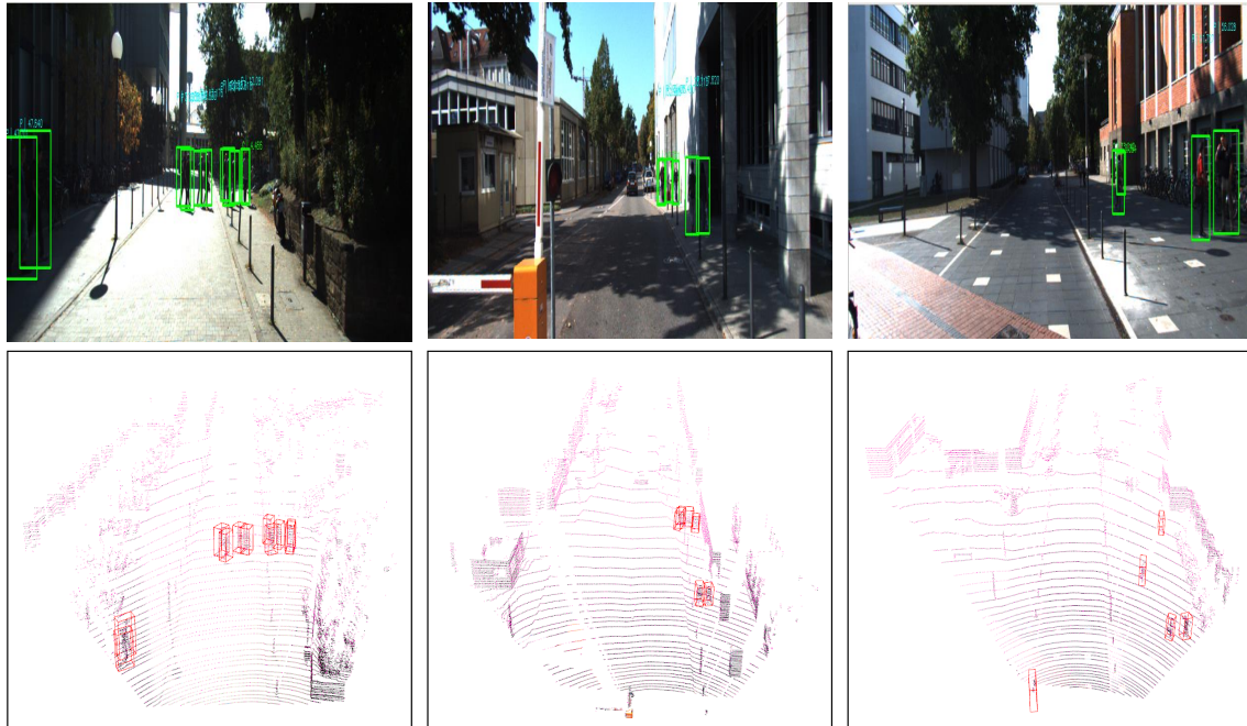
Figure 3.4: Qualitative 3D detection results of our architecture on the Pedestrian category of KITTI test set. The detected objects are shown with red 3D bounding boxes and green 2D bounding boxes. The upper row shows the 2D bounding box in the RGB images and the bottom row shows the results in the corresponding point clouds.
