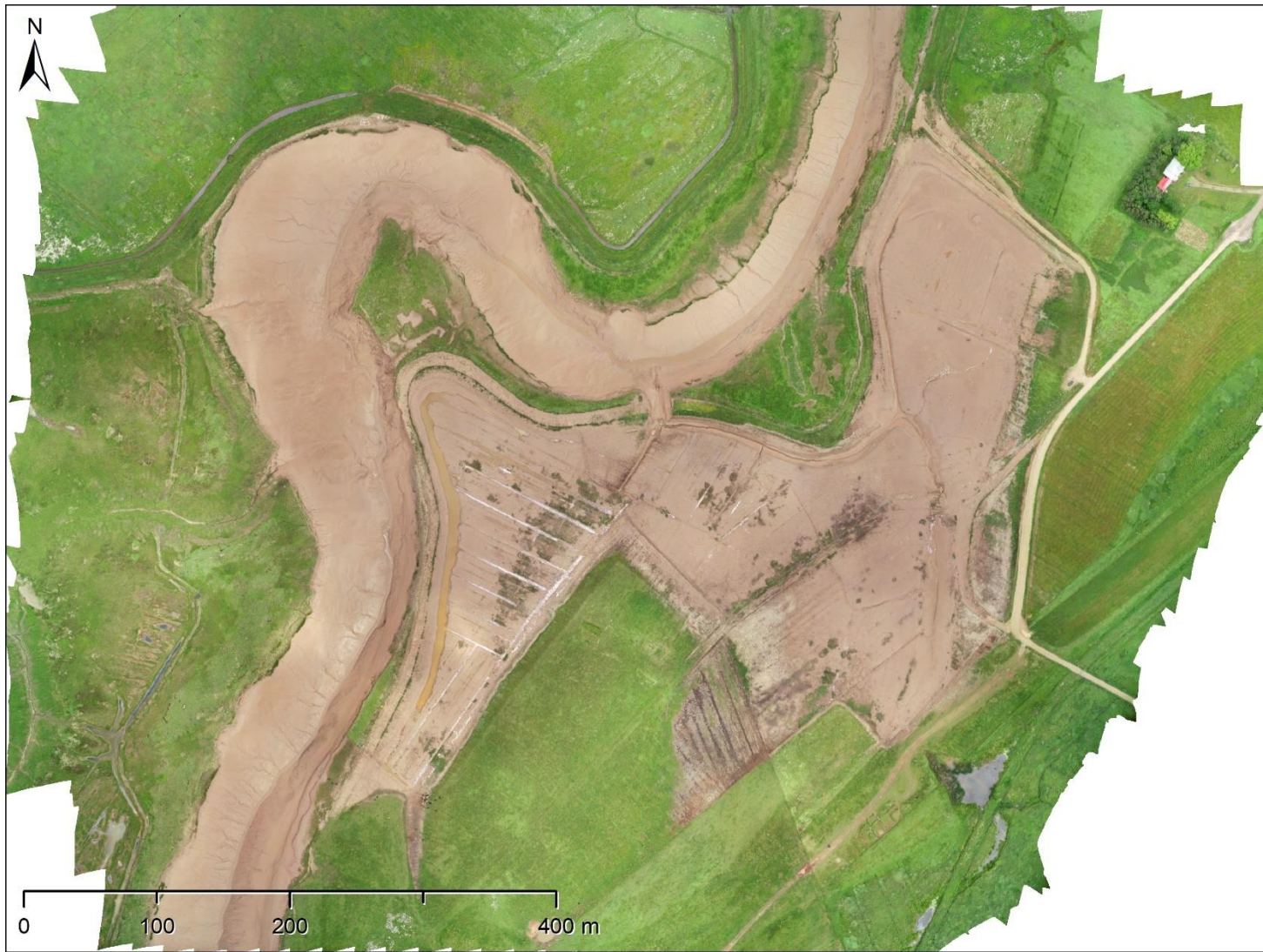
Figure D-5. RGB orthomosaic produced by Agisoft Metashape. Imagery data collected with a DJI Phantom 4 RTK RPAS during a full site survey of Converse, July 9, 2020. Resolution is 3.5cm and horizontal RMSE expected to be less than the resolution.
