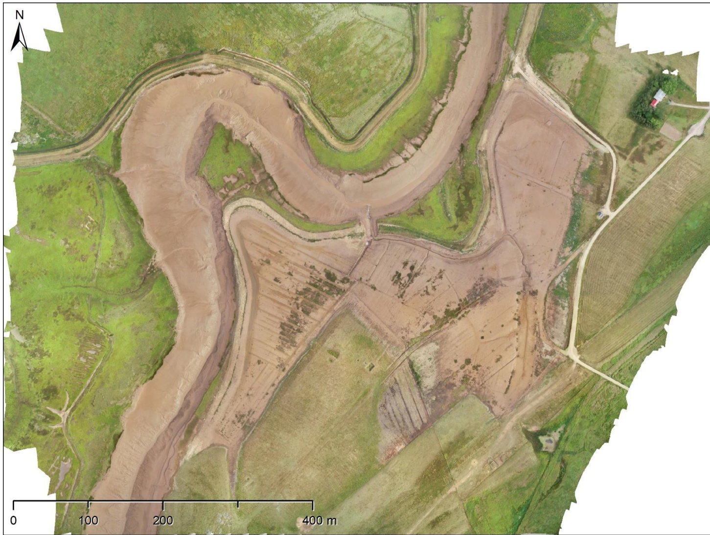
Figure D-7. RGB orthomosaic produced by Agisoft Metashape. Imagery data collected with a DJI Phantom 4 RTK RPAS during a full site survey of Converse, August 21, 2020. Resolution is 3.5cm and horizontal RMSE expected to be less than the resolution.
