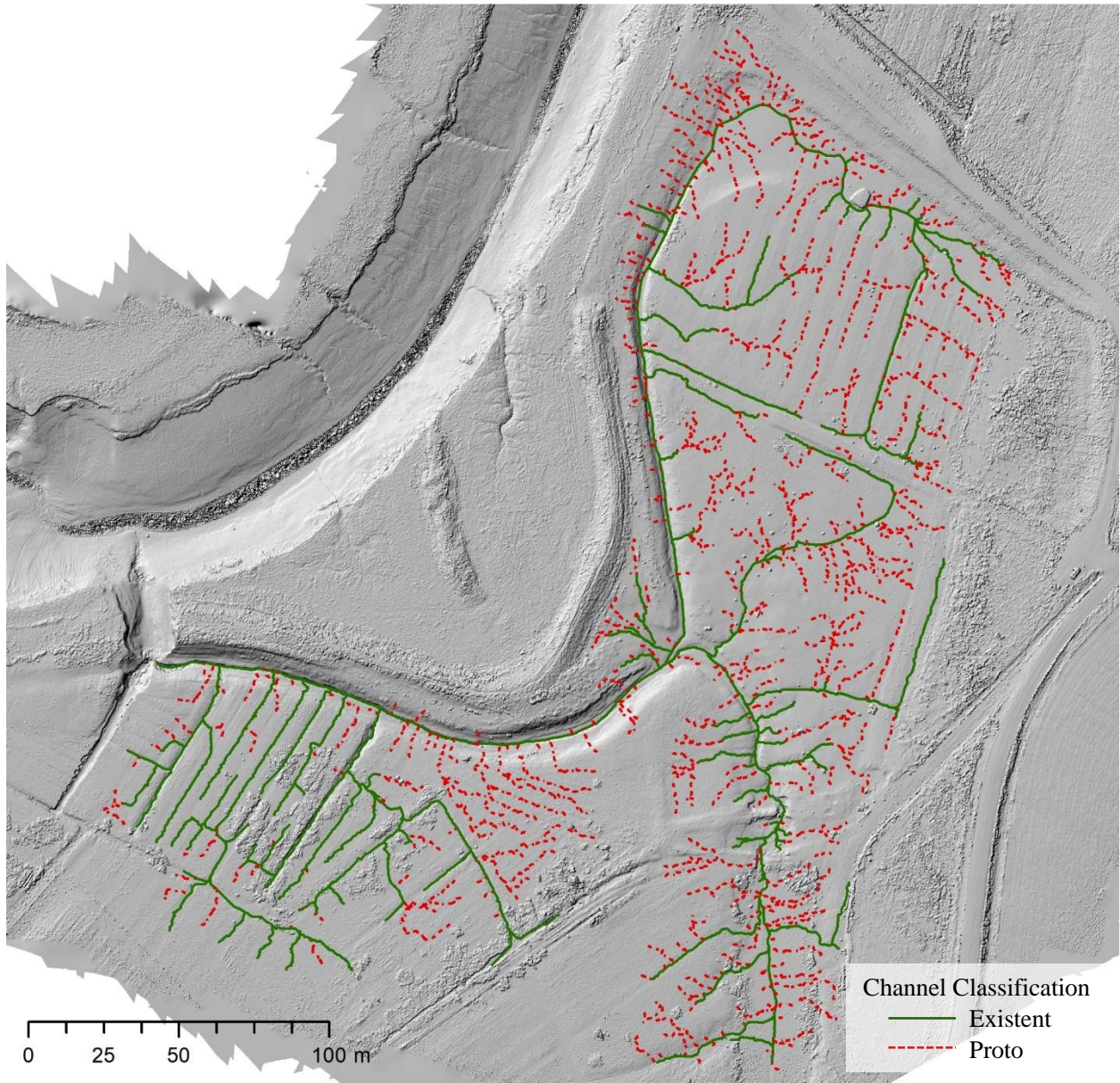
Figure G-12. Results of the channel delineation of the November 8, 2020 Target Area dataset.
