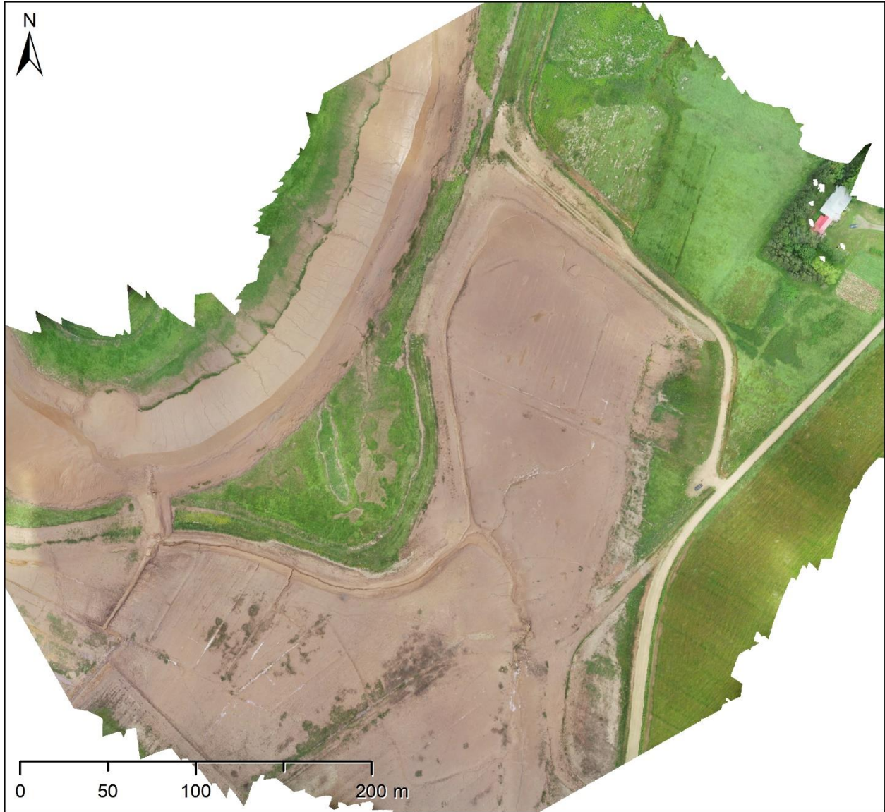
Figure E-5. RGB orthomosaic produced by Agisoft Metashape. Imagery data collected with a DJI Phantom 4 RTK RPAS during a target area survey of Converse, July 9, 2020. Resolution is 2 cm and horizontal RMSE expected to be less than the resolution.
