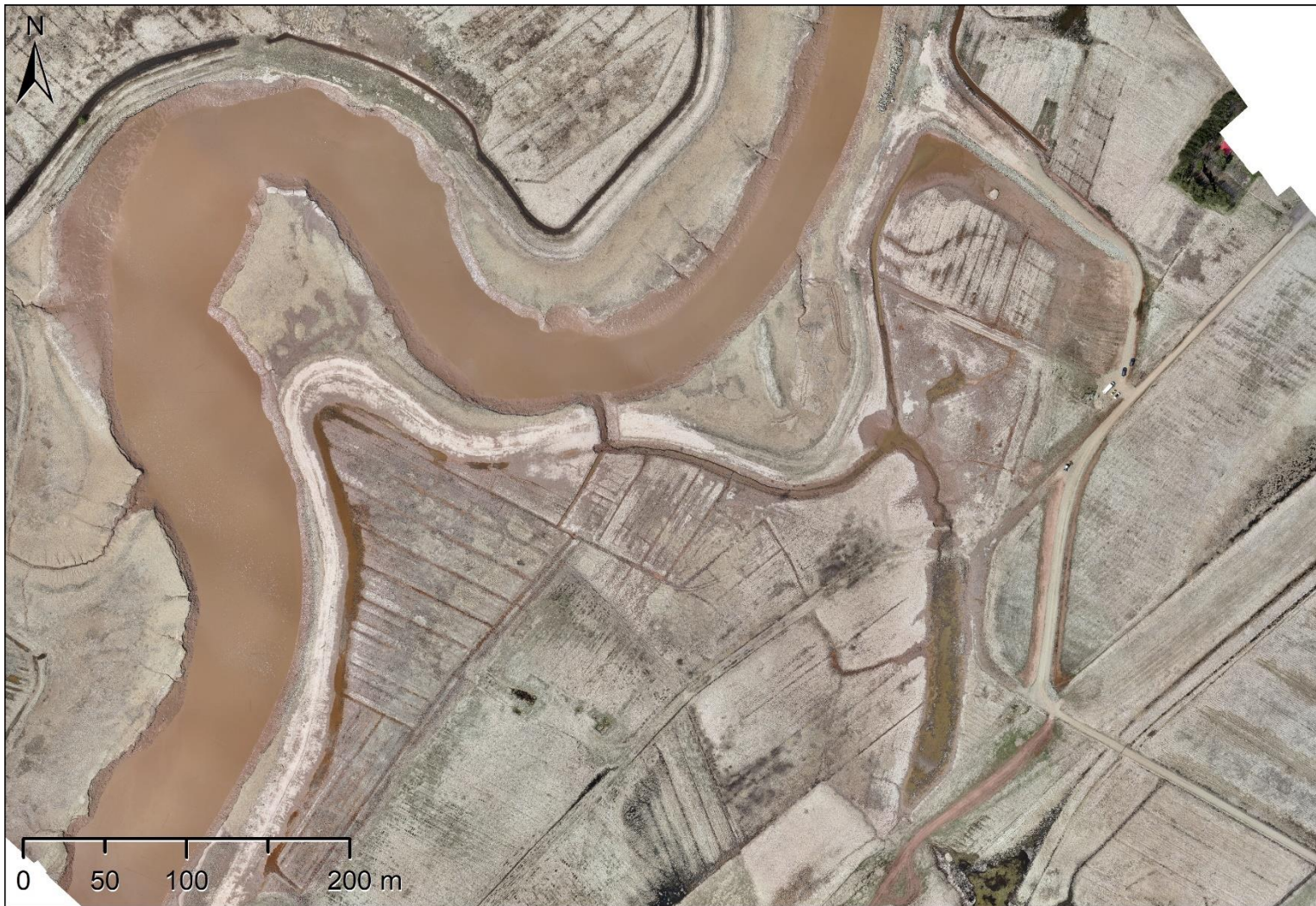
Figure J-5. RGB orthomosaic produced by Pix4DMapper. Imagery data collected with a WingtraOne PPK RPAS during a full site survey of Converse, May 5, 2019. Orthomosaic resolution of 4 cm, and horizontal RMSE expected to be less than the resolution.
