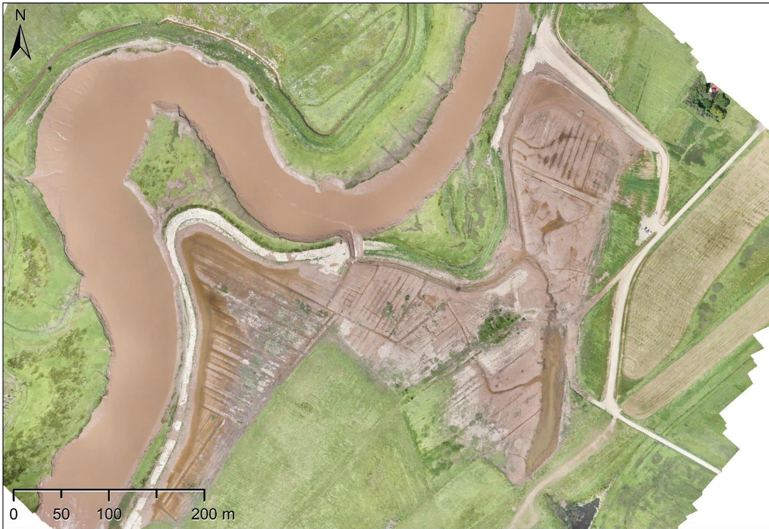
Figure J-7. RGB orthomosaic produced by Agisoft Metashape. Imagery data collected with a WingtraOne PPK RPAS during a full site survey of Converse, August 2, 2019. Orthomosaic resolution of 2.5 cm, and horizontal RMSE expected to be less than the resolution.
