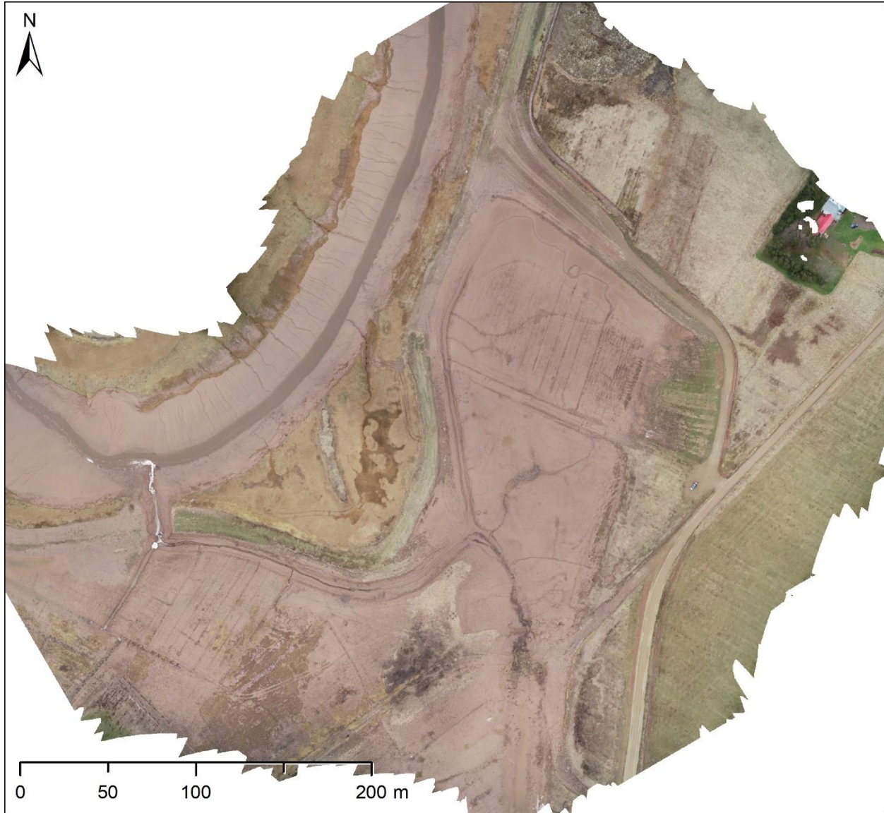
Figure E-1. RGB orthomosaic produced by Agisoft Metashape. Imagery data collected with a DJI Phantom 4 RTK RPAS during a target area survey of Converse, November 24, 2019. Resolution is 2 cm and horizontal RMSE expected to be less than the resolution.
