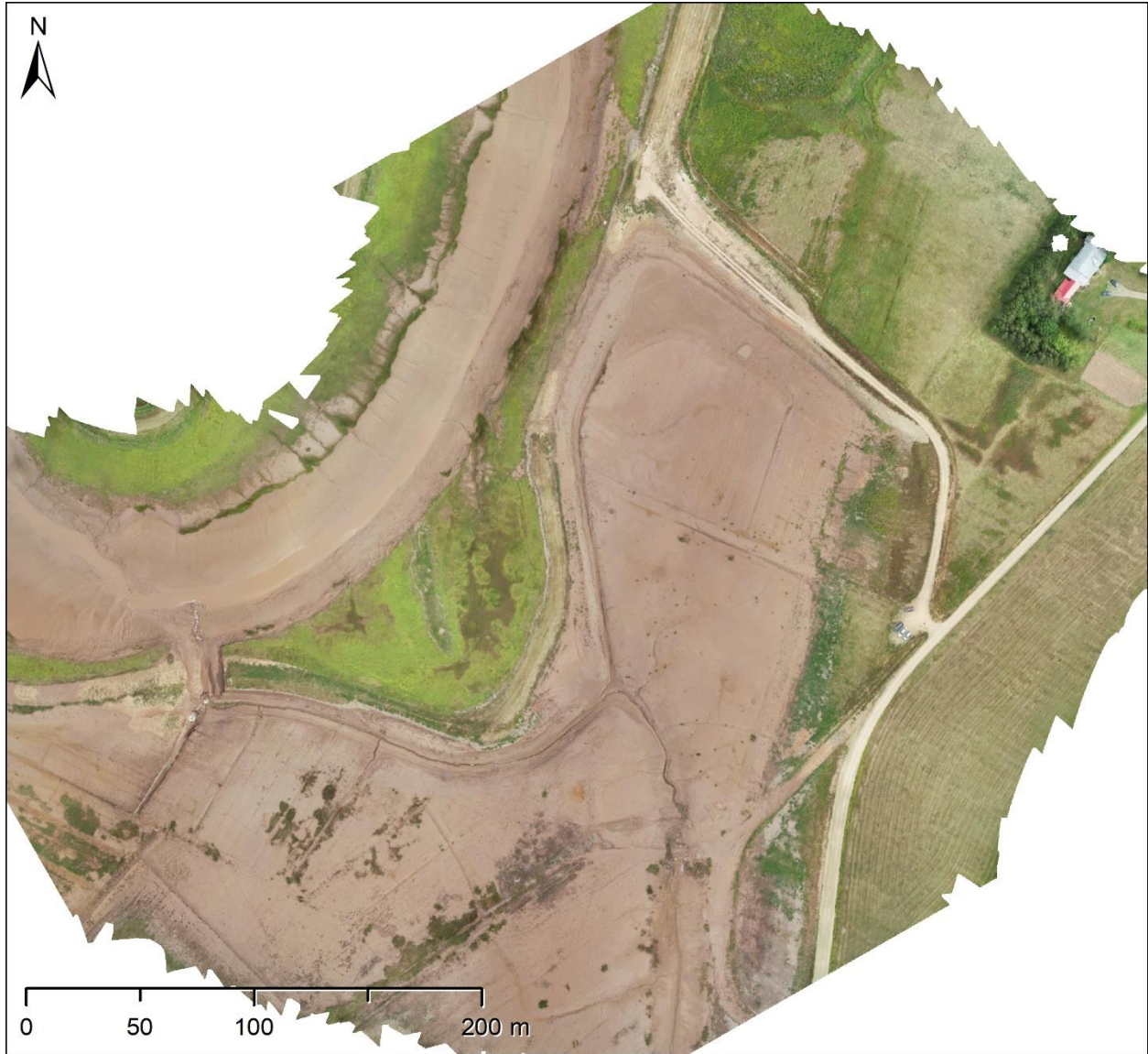
Figure E-7. RGB orthomosaic produced by Agisoft Metashape. Imagery data collected with a DJI Phantom 4 RTK RPAS during a target area survey of Converse, August 21, 2020. Resolution is 2 cm and horizontal RMSE expected to be less than the resolution.
