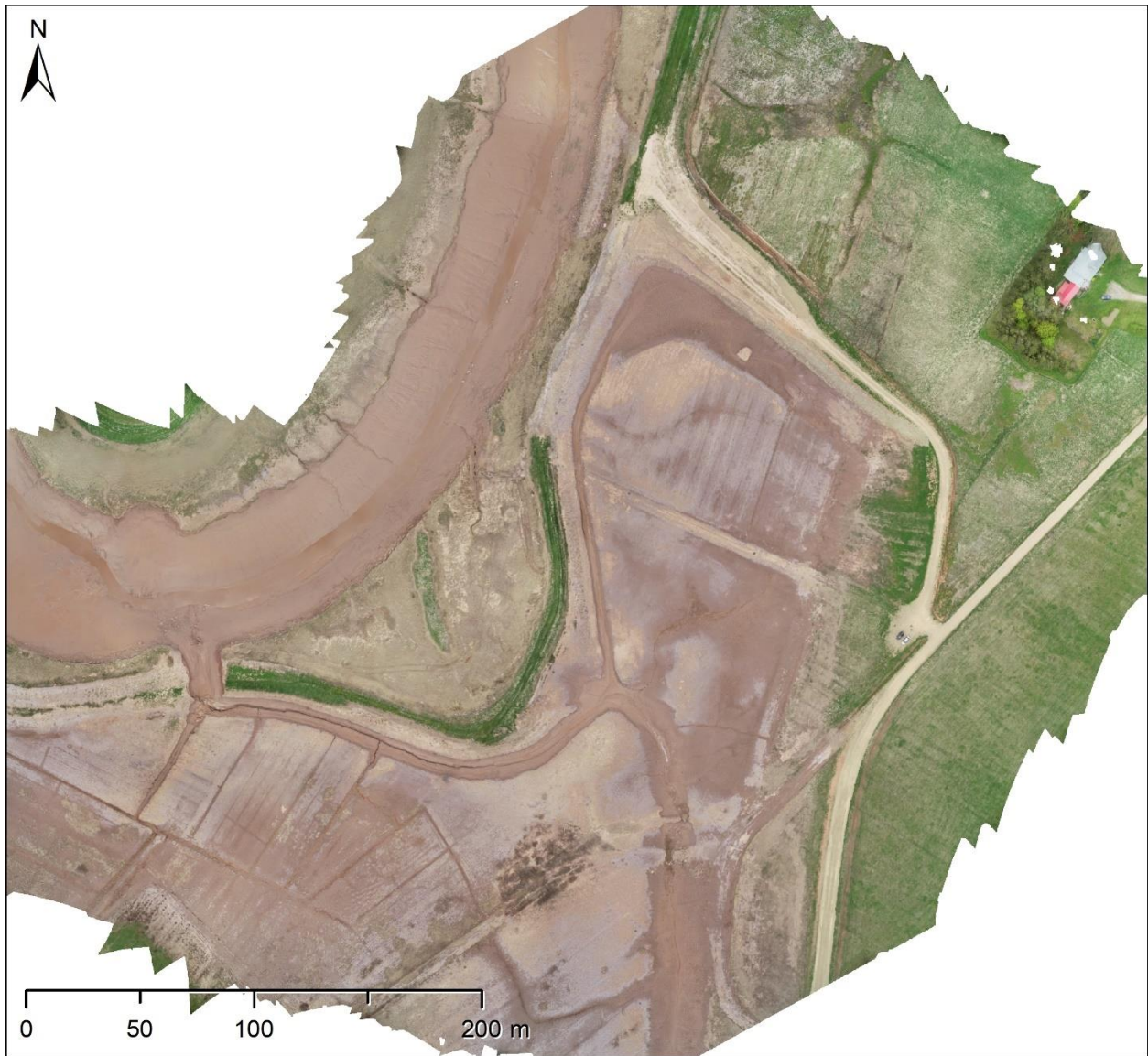
Figure E-3. RGB orthomosaic produced by Agisoft Metashape. Imagery data collected with a DJI Phantom 4 RTK RPAS during a target area survey of Converse, June 1, 2020. Resolution is 2 cm and horizontal RMSE expected to be less than the resolution.
