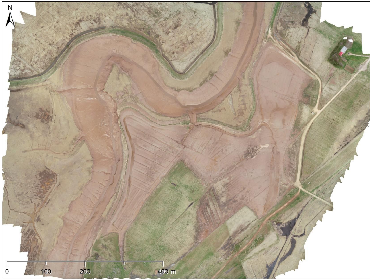
Figure D-13. RGB orthomosaic produced by Agisoft Metashape. Imagery data collected with a DJI Phantom 4 RTK RPAS during a full site survey of Converse, May 4, 2021. Resolution is 3.5cm and horizontal RMSE expected to be less than the resolution.
