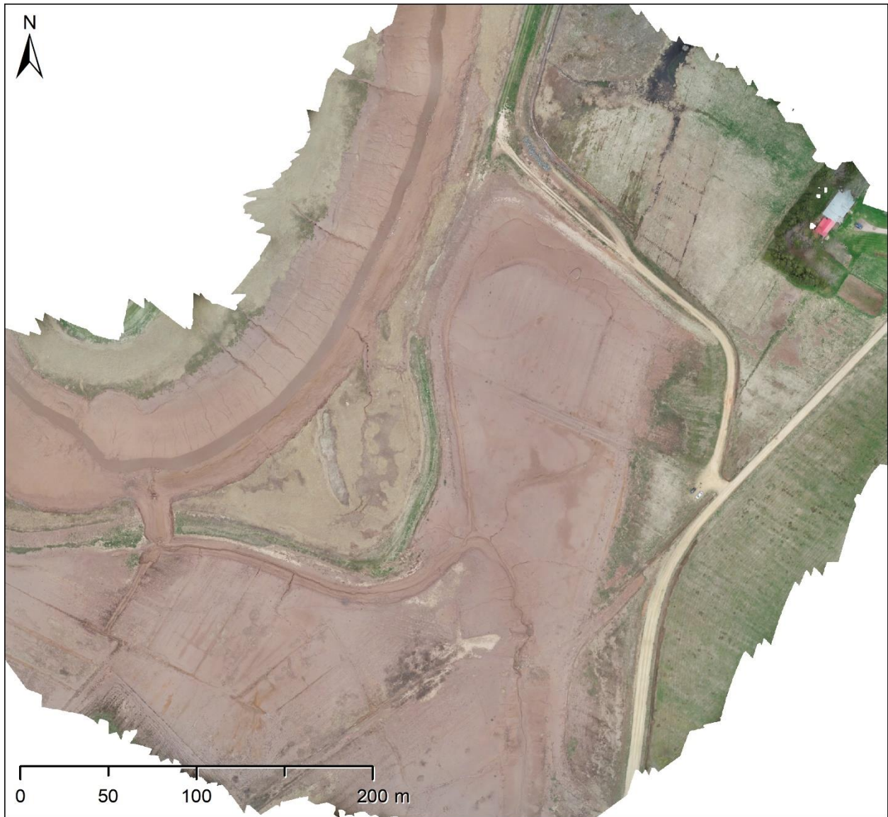
Figure E-13. RGB orthomosaic produced by Agisoft Metashape. Imagery data collected with a DJI Phantom 4 RTK RPAS during a target area survey of Converse, May 4, 2021. Resolution is 2 cm and horizontal RMSE expected to be less than the resolution.
