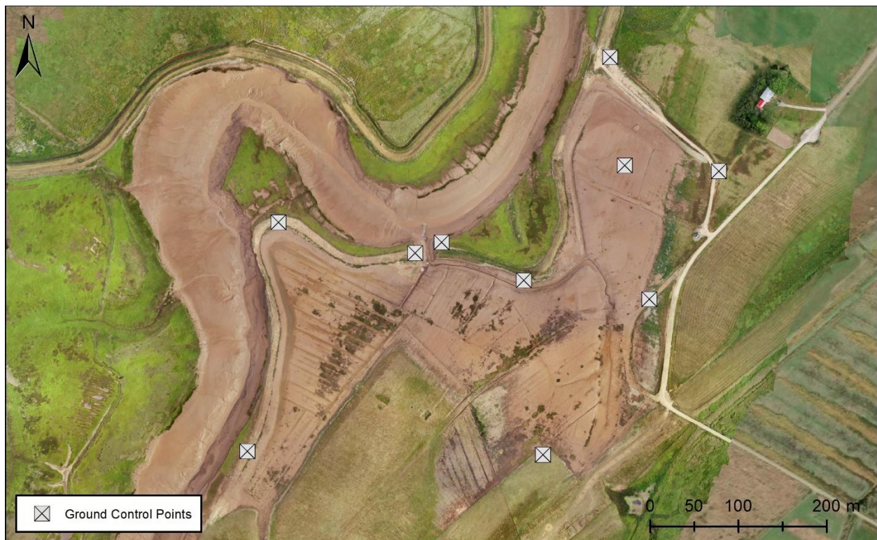
Figure 3.3. Approximate GCP deployment locations at the Converse restoration site for RPAS aerial surveys. GCP locations varied slightly between deployments. Background imagery collected August 21, 2020 with a DJI Phantom 4 RTK RPAS.
