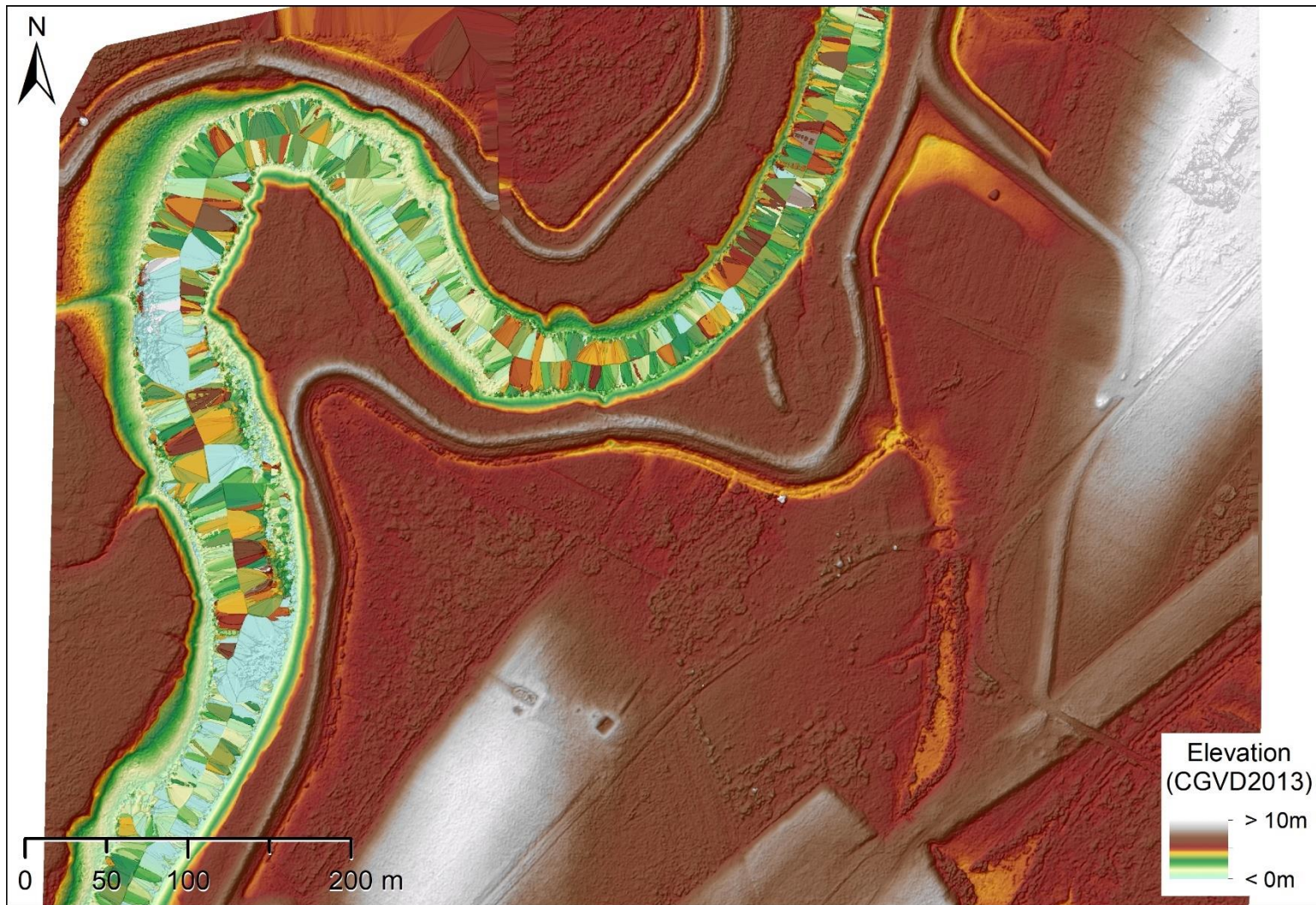
Figure J-4. Elevation model produced by Pix4D Mapper. Imagery data collected with a DJI Phantom 3 Professional RPAS during a full site survey of Converse, September 24, 2018, pre-breach. Elevation model resolution of 4 cm, and vertical RMSE of 15.7 cm.
