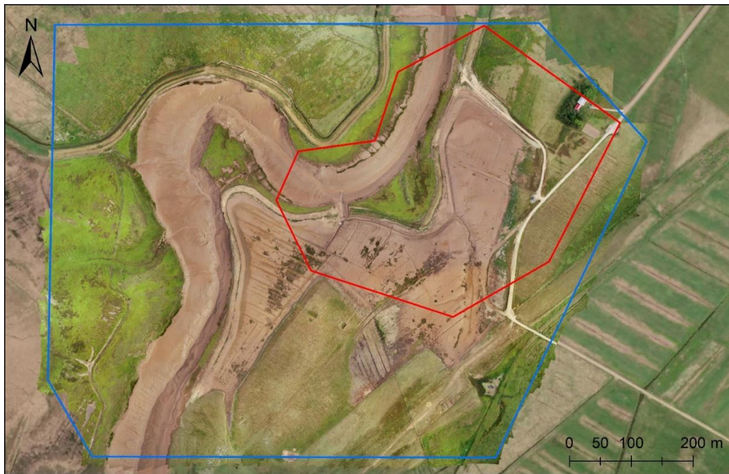
Figure 3.2. Approximate coverage of each flight type, full site (blue polygon) and target area (red polygon) for RPAS aerial surveys of the Converse restoration site. Background imagery collected August 21, 2020 with a DJI Phantom 4 RTK RPAS.
