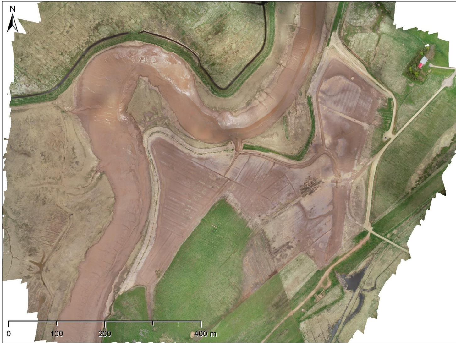
Figure D-3. RGB orthomosaic produced by Agisoft Metashape. Imagery data collected with a DJI Phantom 4 RTK RPAS during a full site survey of Converse, June 1, 2020. Resolution is 3.5cm and horizontal RMSE expected to be less than the resolution.
