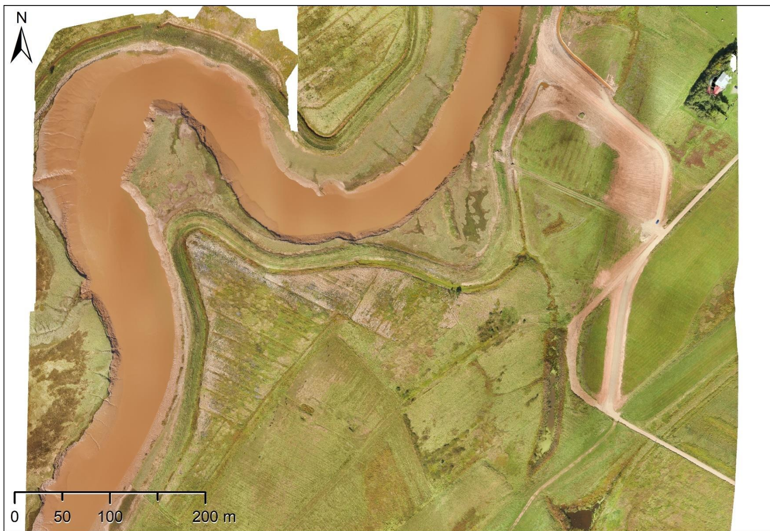
Figure J-3. RGB orthomosaic produced by Pix4D Mapper. Imagery data collected with a DJI Phantom 3 Professional RPAS during a full site survey of Converse, September 24, 2018, pre-breach. Orthomosaic resolution of 4 cm, and horizontal RMSE expected to be less than the resolution.
