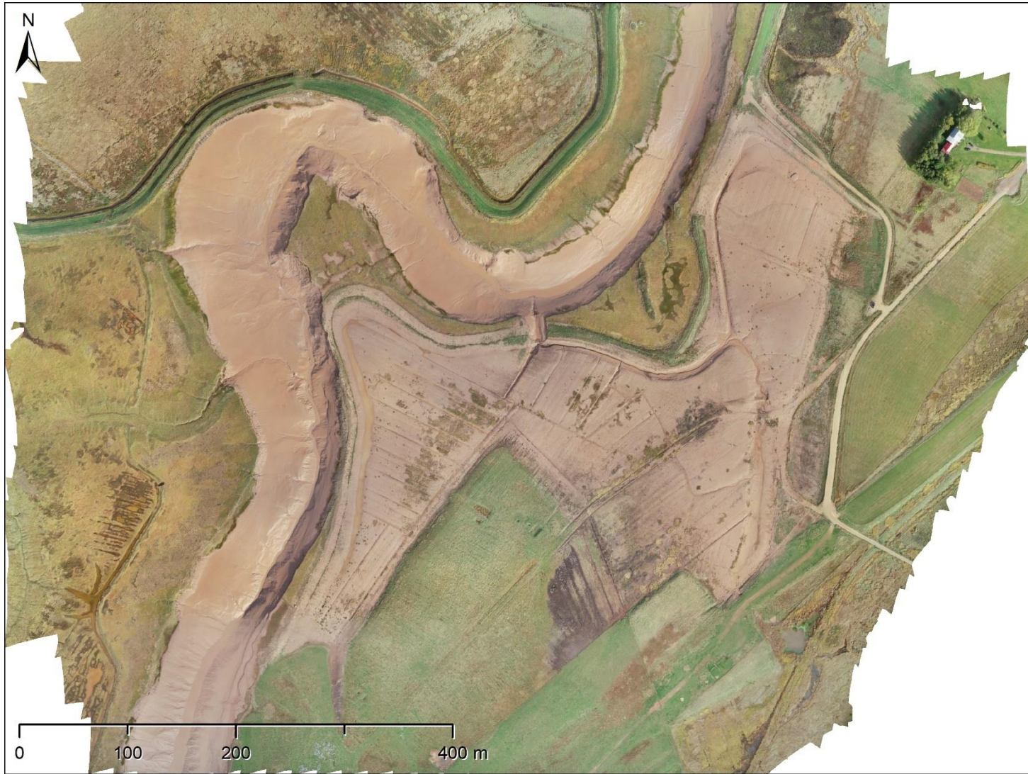
Figure D-9. RGB orthomosaic produced by Agisoft Metashape. Imagery data collected with a DJI Phantom 4 RTK RPAS during a full site survey of Converse, October 5, 2020. Resolution is 3.5cm and horizontal RMSE expected to be less than the resolution.
