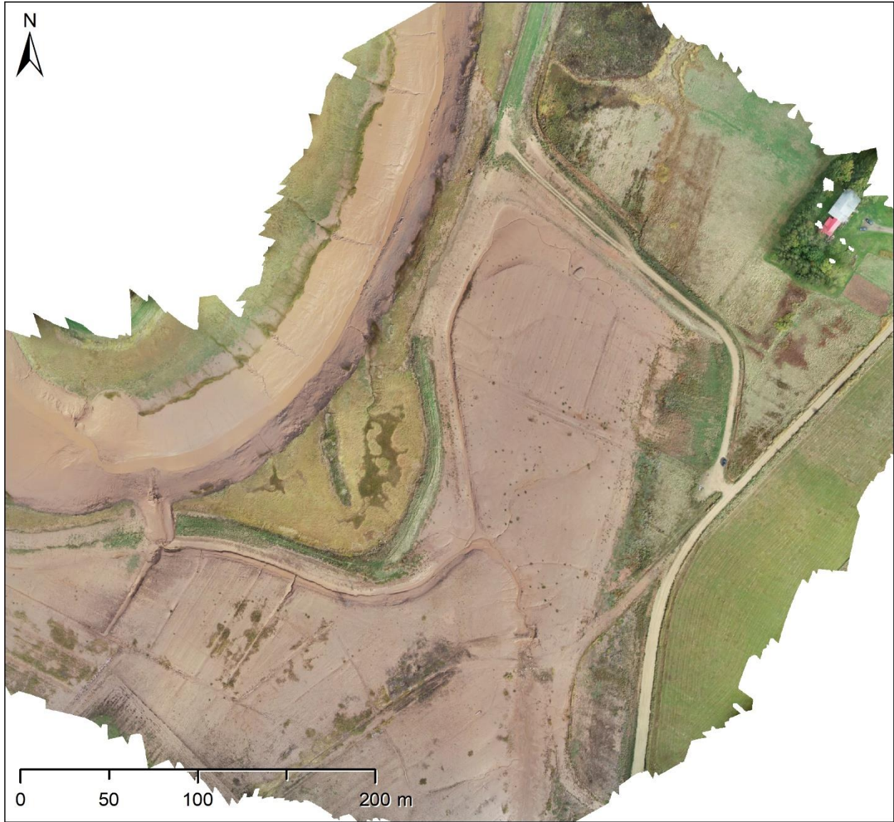
Figure E-9. RGB orthomosaic produced by Agisoft Metashape. Imagery data collected with a DJI Phantom 4 RTK RPAS during a target area survey of Converse, October 5, 2020. Resolution is 2 cm and horizontal RMSE expected to be less than the resolution.
