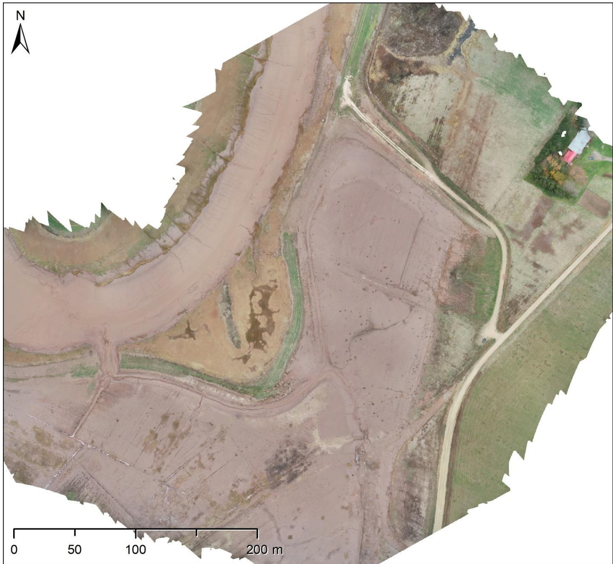
Figure E-11. RGB orthomosaic produced by Agisoft Metashape. Imagery data collected with a DJI Phantom 4 RTK RPAS during a target area survey of Converse, November 8, 2020. Resolution is 2 cm and horizontal RMSE expected to be less than the resolution.
