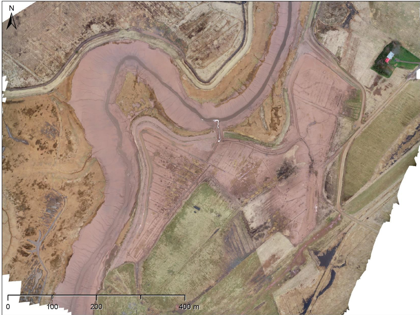
Figure D-1. RGB orthomosaic produced by Agisoft Metashape. Imagery data collected with a DJI Phantom 4 RTK RPAS during a full site survey of Converse, November 24, 2019. Resolution is 3.5cm and horizontal RMSE expected to be less than the resolution.
