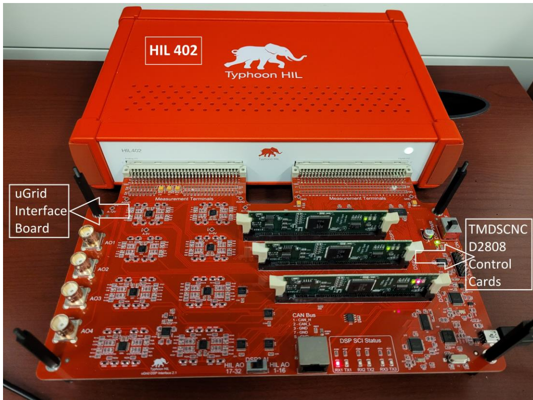
Figure 4.8: The C-HIL testbed, including the HIL402 device, control cards, and interface boards
