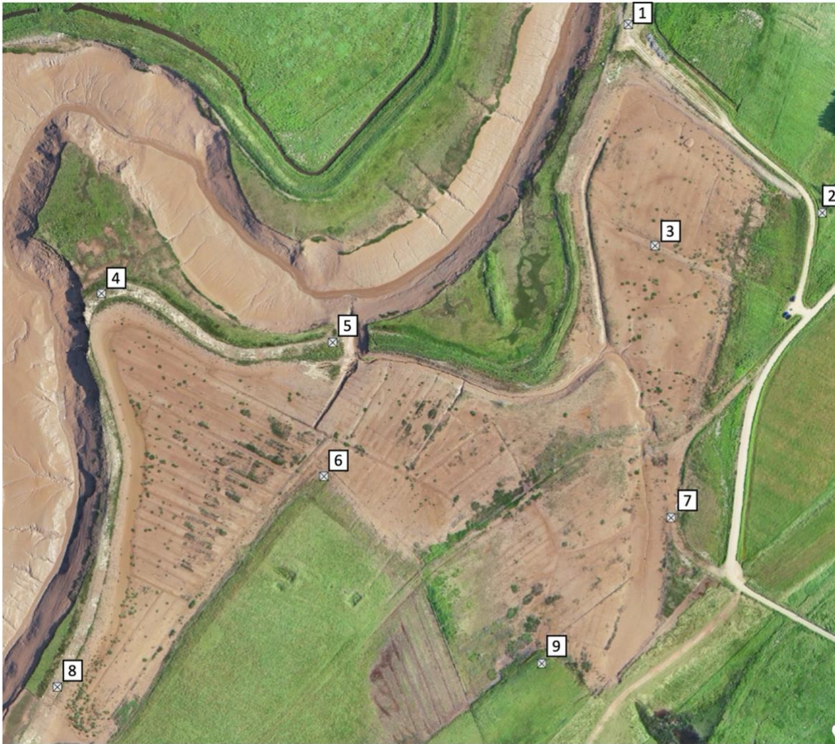
Figure 3.6. Approximate GCP deployment locations (n=9) at the Converse restoration site for the RPAS aerial survey. Background imagery collected July 25, 2021, with a DJI Phantom 4 RTK RPAS by CBWES Inc.
