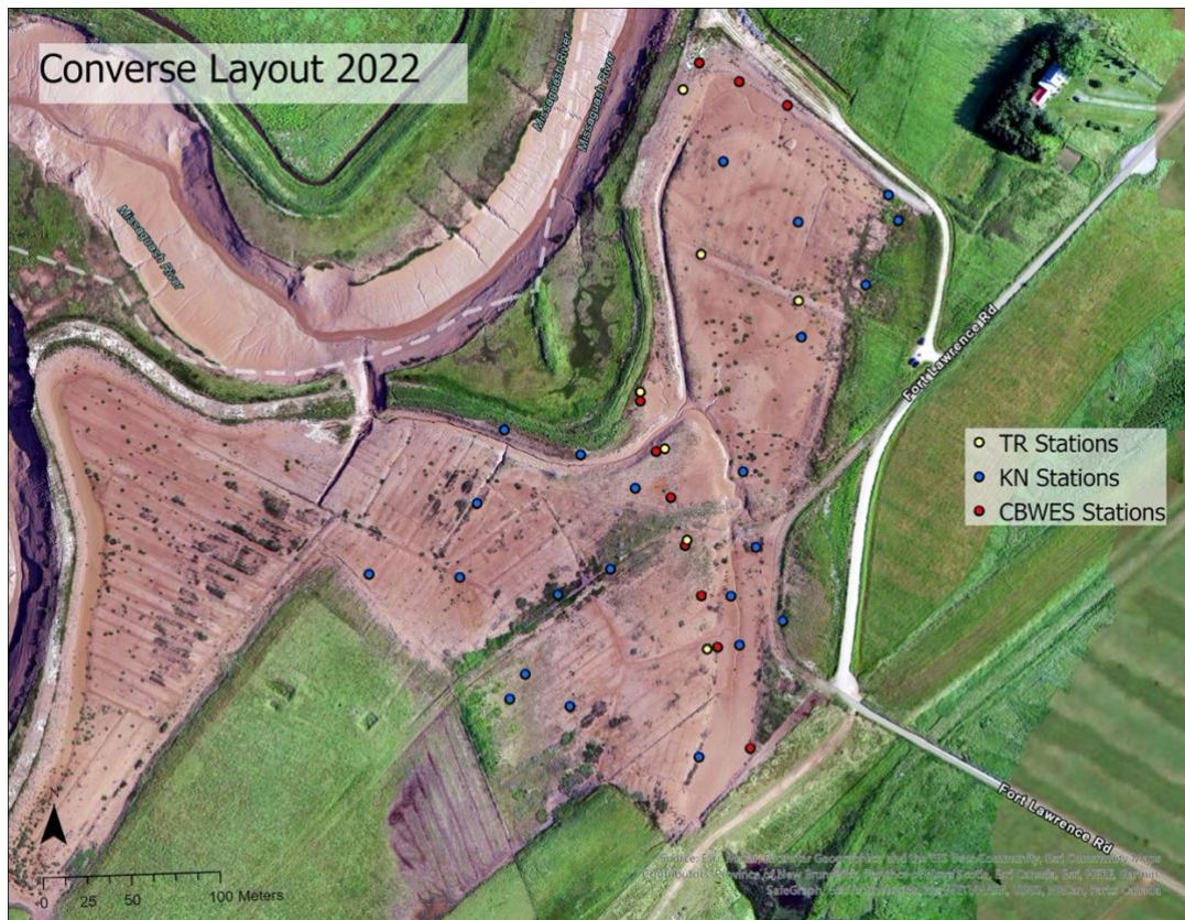
Figure 3.3. Final sampling station locations (n=40) for field data collection. Background imagery collected July 25, 2021, by CBWES with a DJI Phantom 4 RTK RPAS.
