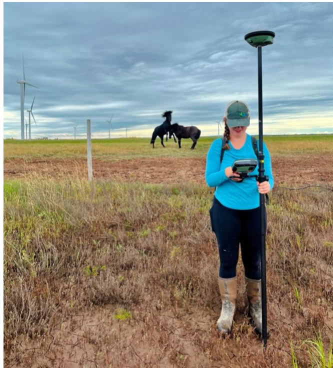
Figure 3.4. Measuring the location and elevation of survey stations using a Leica GS14 RTK GNSS unit on August 2, 2022. (Credit: TransCoastal Adaptations).
