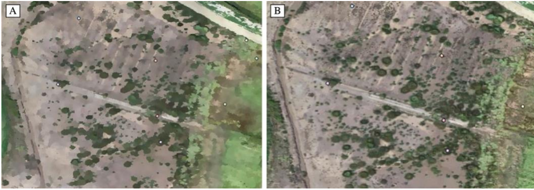
Figure 3.7. Screenshot of the result of changing the spectral detail in the image segmentation process: A) spectral detail = 15.00; B) spectral detail = 20.00.
