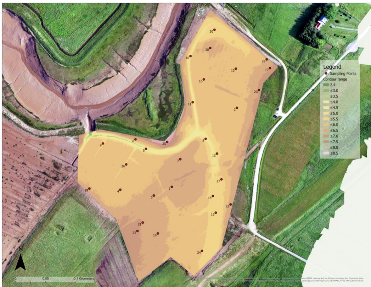
Figure 3.2. Sampling stations (n=30) placed within 13 different elevation bins at the Converse restoration site. Background imagery collected July 25, 2021 with a DJI Phantom 4 RTK RPAS.
