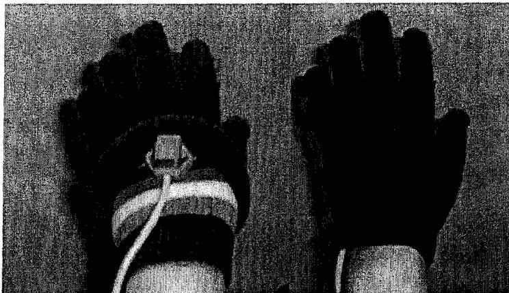
Figure 3.1: Polhemus 3D motion capture sensors are attached to the gloves. (Only the left hand is shown)
