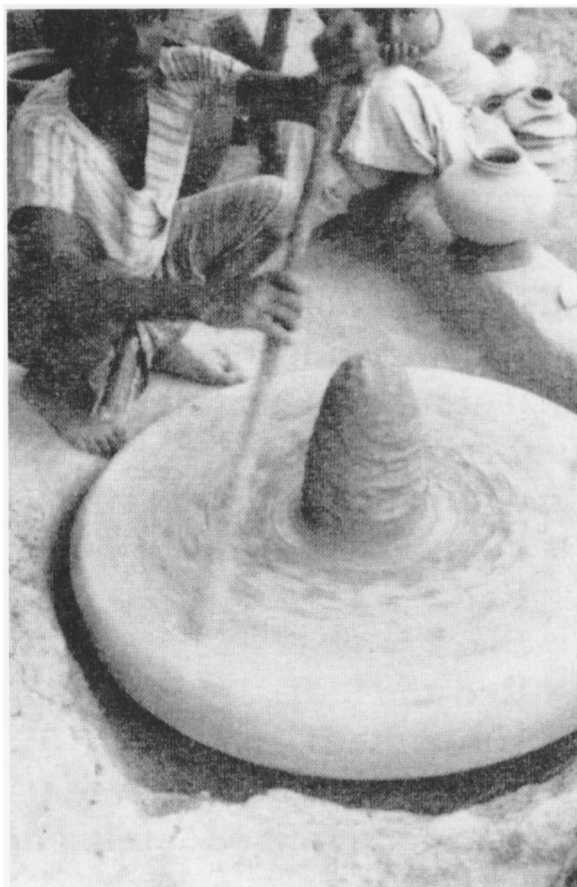
Fig. 6. Potter using a rod to bring a single-wheel type potter's wheel up to throwing speed. Dangwara, India (Miller 1985, fig. 61b; © Cambridge University Press).
