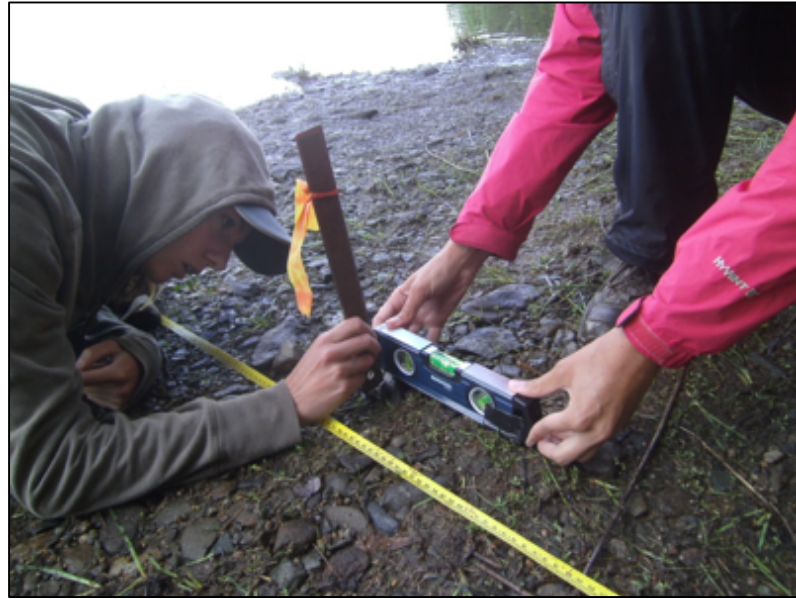
Figure 4-3. Picture showing fine scale elevation measurement with a level and a ruler along the lakeshore-to-forest gradient.
