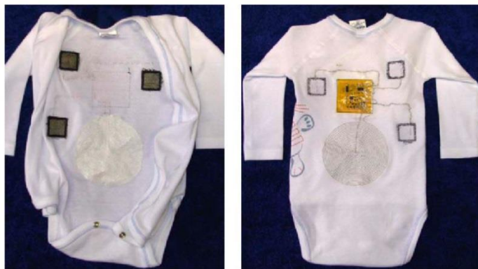
Figure 2.2.2: Baby garment prototype for ECG measurement. (Left) inside showing the textrodes; (right) outside reproduced with permission. 38
