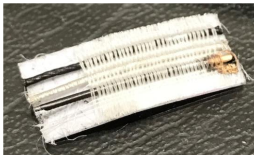
Figure 5.4.2: Achira Labs fabric-based electrode modified with three layers of AgNPs (2 \mu L per layer).
