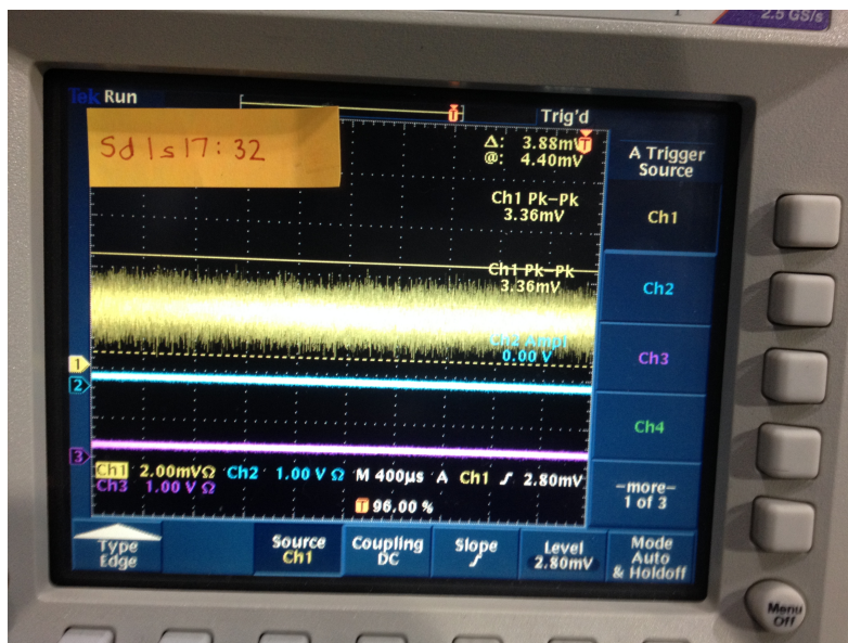
FIGURE 3.10: Electronic noise from (a) YY1 detector's channel (b) S3d1 detector's channel.
