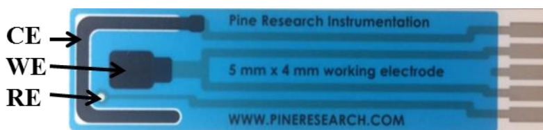
Figure 2.1.1: Labeled SPE, which was used as the EC-SERS substrate in this thesis work.
