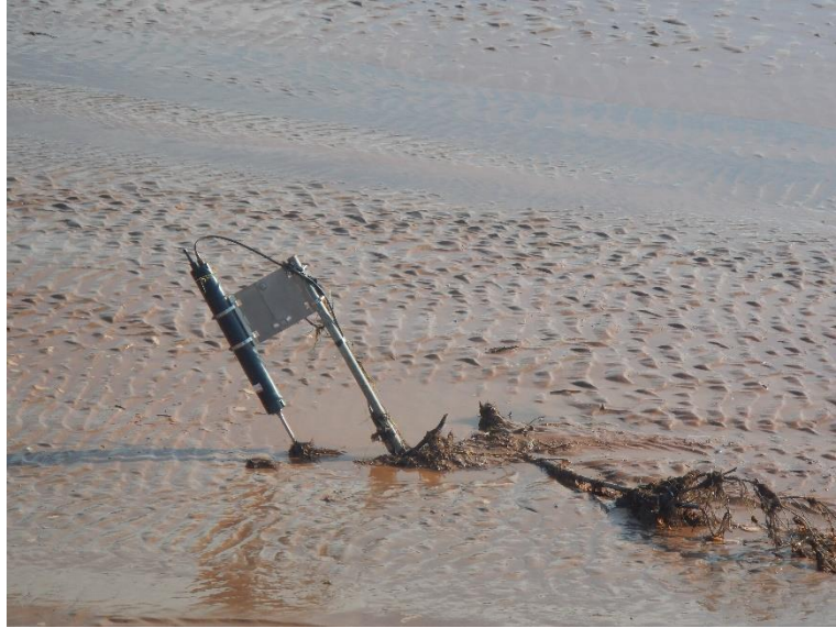
Figure 4.11. ADV 2, and the attached OBS 2, tilted in the upstream direction in the Salmon River at low tide after Tide 1.
