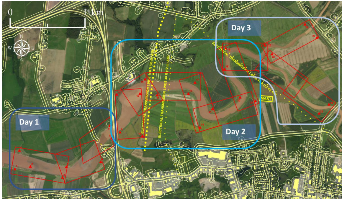
Figure 3.6. Grids flown by an RPA (DJI Phantom ® ) to capture ground elevation of mudflats at low tide. Grids were flown over a span of three days (August 14, August 16 and August 17, 2018). GCPs are numbered and symbolized as red triangles. The red boxes represent each flight grid. Map created by Greg Baker and Reyhan Akyol, MP_SpARC, Saint Mary's University, 2018.
