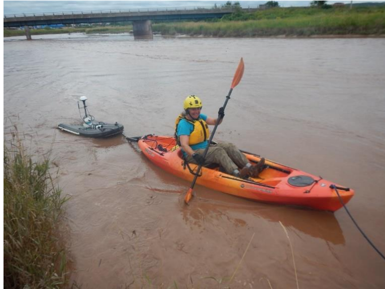
Figure 3.3. The HydroSurveyor™ mounted on the HydroBoard being towed by a kayak in the Salmon River.
