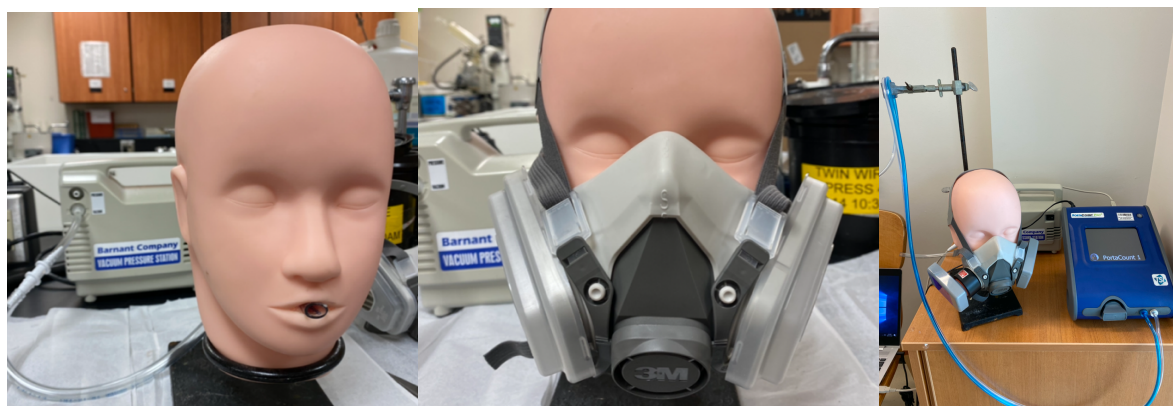
Figure 2-2: The mannequin head set up for aerosol testing.
