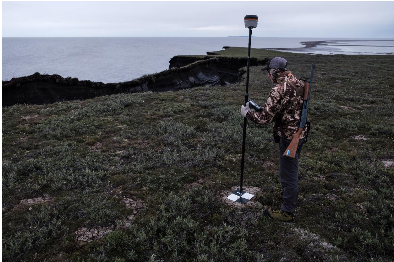
Figure 3.1: A Hemisphere S321 RTK rover being used to collect a GPS point on a GCP on Pelly Islands (August 2018, GSC)
