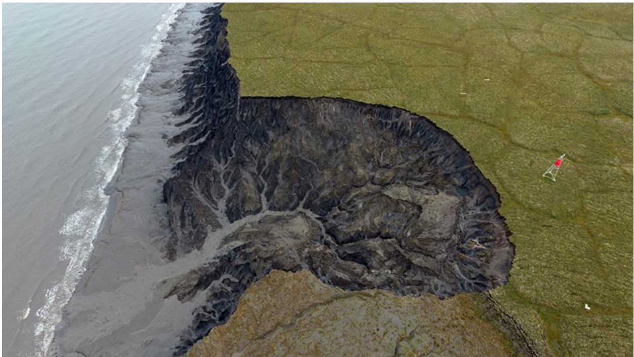
Figure 1.7: Thaw slump along the Canadian Beaufort Sea coast (photo by: Roger Macloed/ 2016 GSC)
