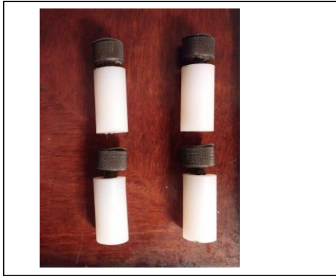
Figure 66. - Four permanent magnets mounted on insulator stubs.
