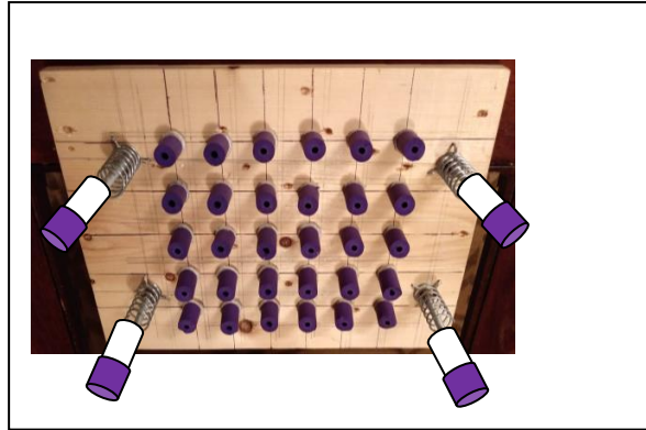
Figure 67. - Screw and spring assembly to attach the permanent magnets.
