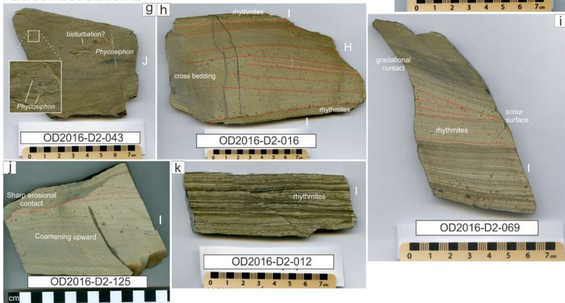
Figure 5.4. Examples of sedimentary structures in lithofacies associations 1 and 2. The facies letter is labelled next to the facies. Sedimentary features are labelled. Sample 123 in (b) shows a variety of sedimentary structures in the same rock.
